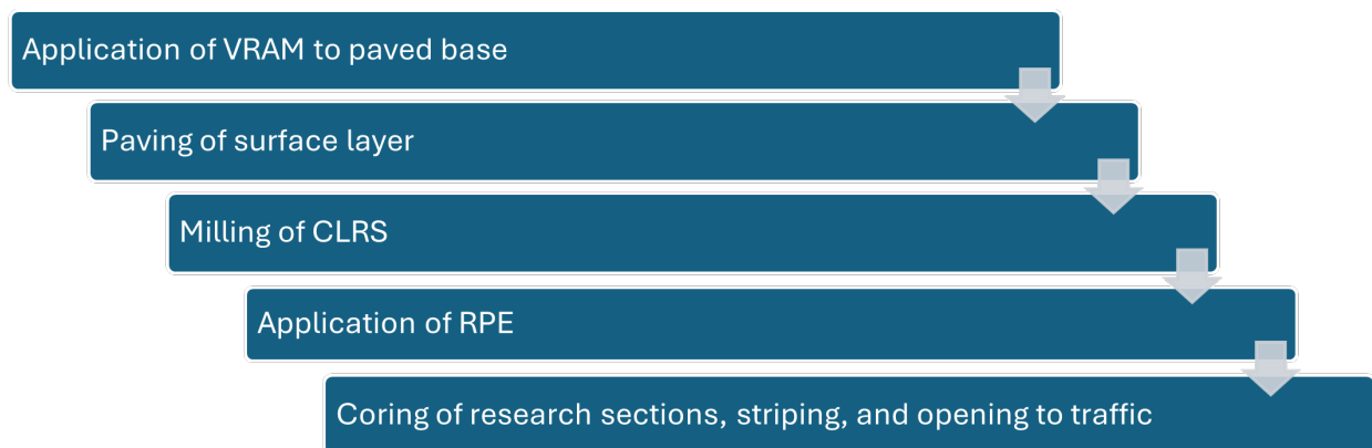
Figure 5.6: Construction Process Sequencing.
