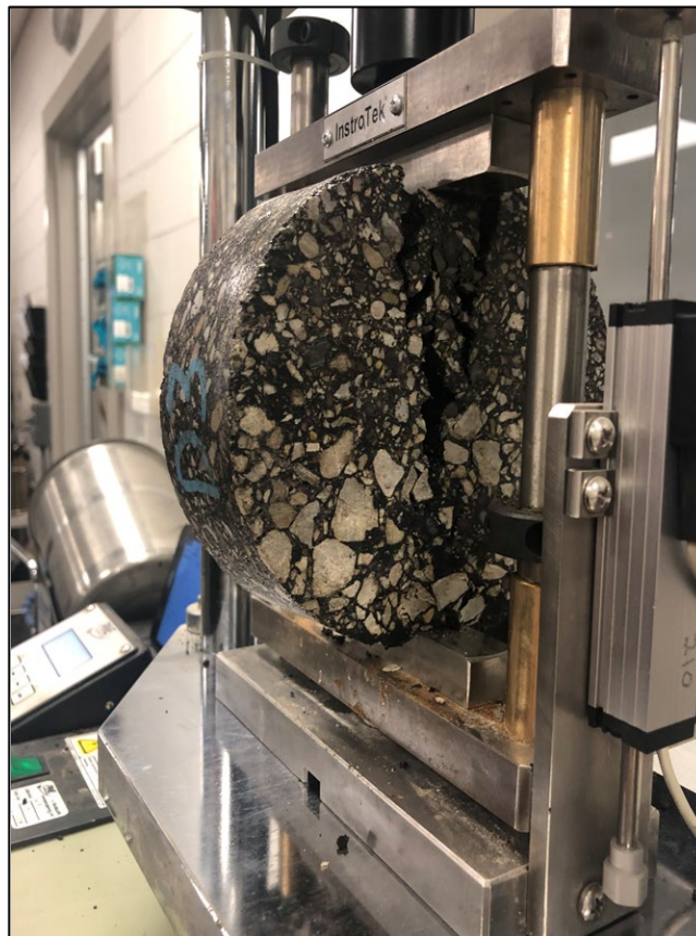
Figure 6.7: IDEAL-CT Setup for Testing of Field Cores.
