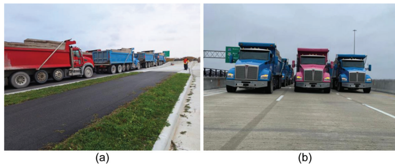
Figure 2.15 Photographs of the trucks taken during the live load test on the Whitestown Parkway Bridge: (a) side view, and (b) front view.
