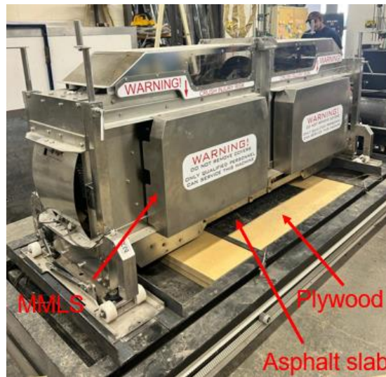
Figure 12. MMLS test setup with restrained asphalt slab.
