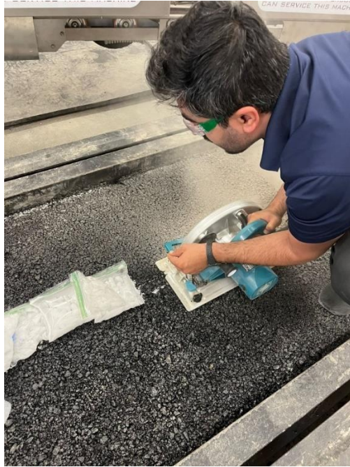
Figure 14. Cutting asphalt slab.
