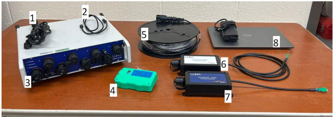
Figure 1. OdiSI 6104 sensor interrogator components: (1) ODiSI power cord, (2) USB3 type A-to-B cable, (3) sensor interrogator, (4) fiber cleaner, (5) standoff cable, (6) extended length remote module, (7) standard length remote module, and (8) instrument controller (laptop computer).
