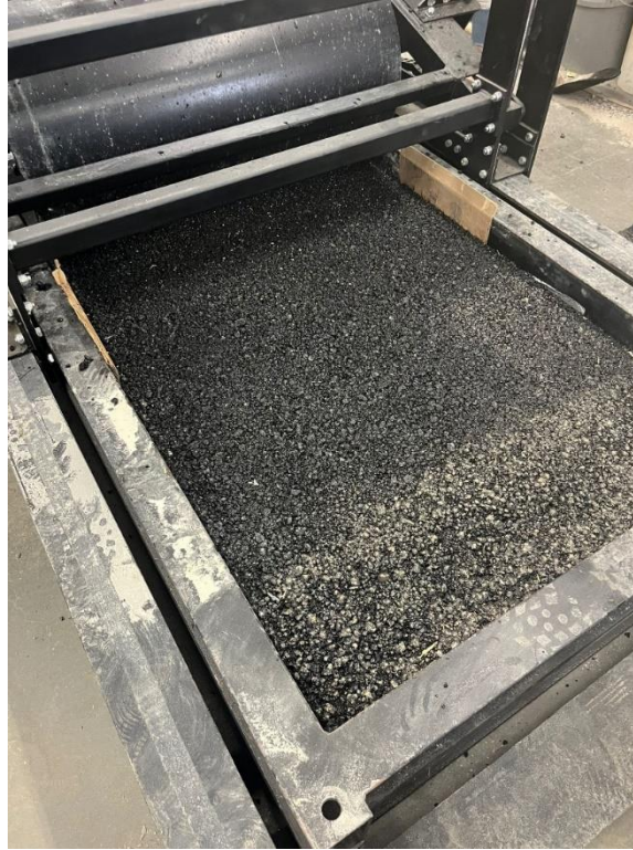
Figure 13. Asphalt slab compaction using MMLS drum roller.
