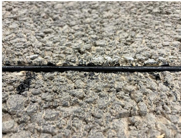
Figure 28. Embedment of strain fiber optic cable into asphalt.
