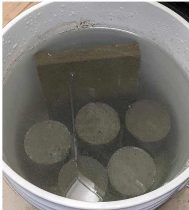
Demolded Concrete specimen kept in water tank to cure
