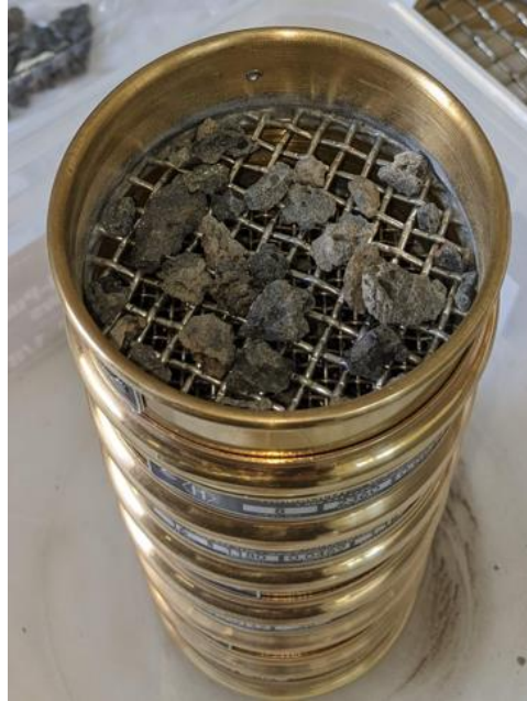
Stacked sieves arranged in descending mesh size containing a geological sample for particle size analysis
