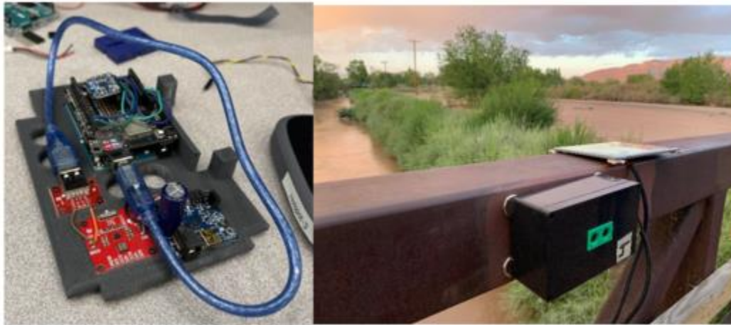
Figure 7. LEWIS sensor: Components (left) and in-field inspection setup (right), demonstrating its application for structural monitoring.
