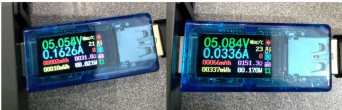
Figure 30. The setup used for measuring the amperage and voltage of the batteries during the testing process. On the left is the maximum power drawn in amps while performing networking operations during awake mode. On the right is the power drawn in amps during the sleep mode.
