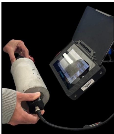
Figure 43. 100BCSA-ECC being tested with ultrasonic velocity device.
