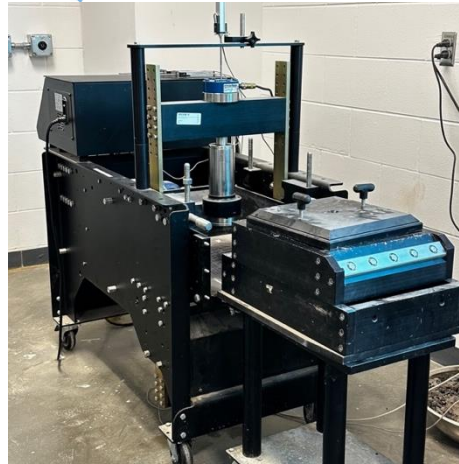
Figure 1: Large-scale direct shear test apparatus
