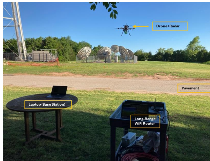
Figure 23 : First test flight with the active integrated payload, taking samples of the road to ensure functionality.
