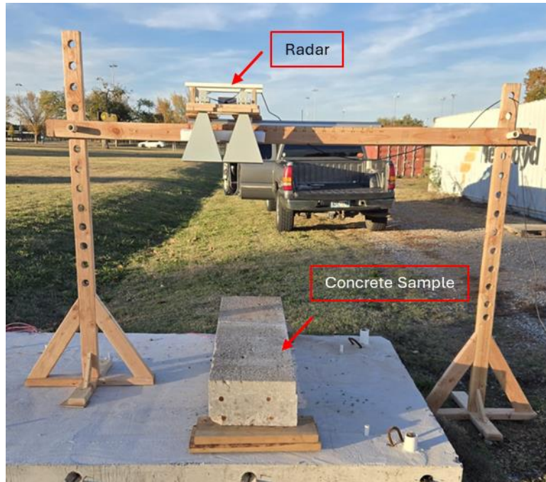
Figure 21 : Concrete block setup and measurement (OU-Fears Lab).
