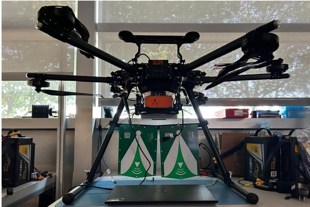
Figure 24 : The second payload configuration with TSA900 antennas in the same plane is mounted under the cargo rack, while the AC power supply and compact processing computer are mounted on the front of the cargo rack, with the radar enclosure placed directly behind.
