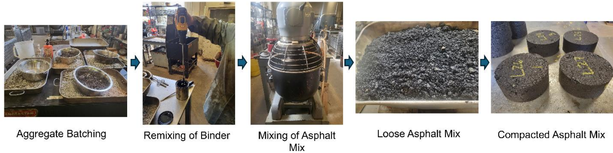
Figure 12. Preparation of asphalt mixes with lignin-modified binder
