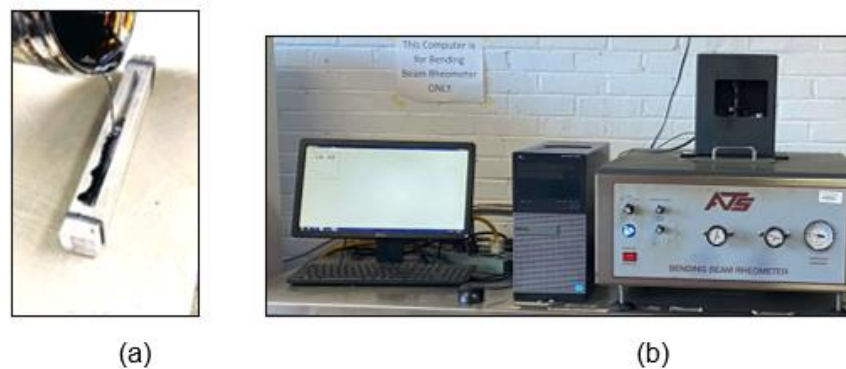
Figure 7. Bending Beam Rheometer (BBR) test: (a) sample preparation and (b) test device
