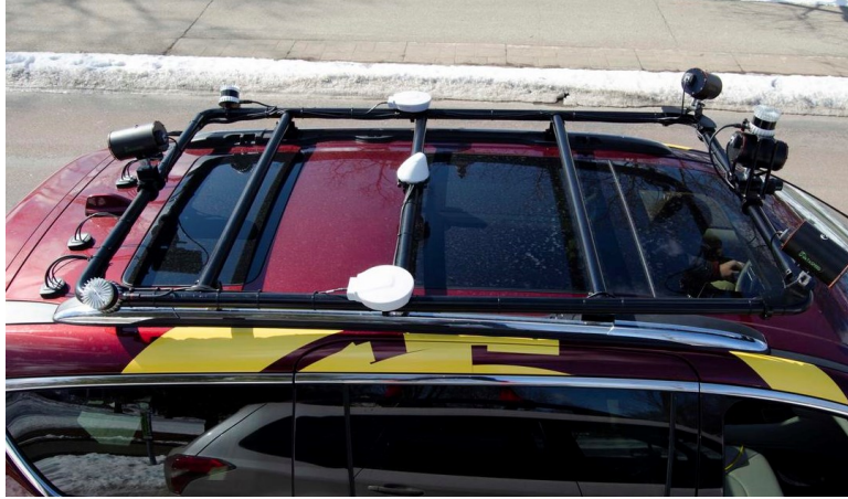
(b) MnCAV vehicle with roof-equipped dual GNSS antenna system
