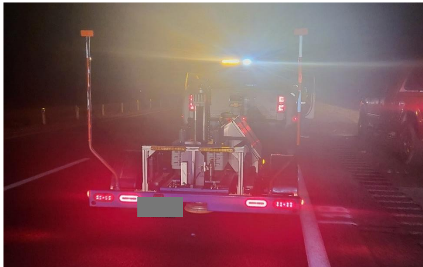
Figure 10 FFWD data collection on I-35 test section
