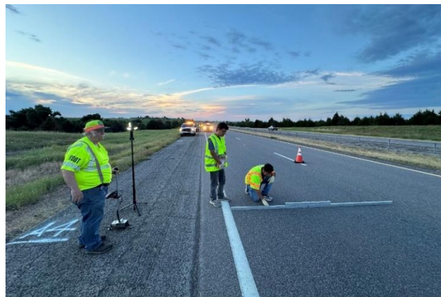
Figure 12 Face Dipstick Measurements on I-35 Test Site
