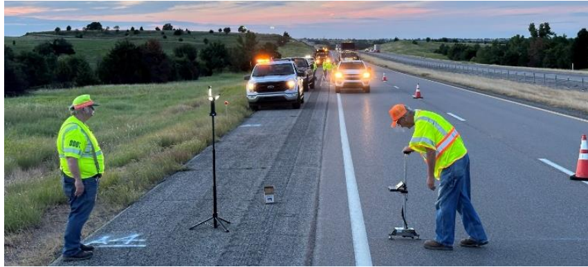
Figure 13 Roadway Profile Measurement using Face Dipstick
