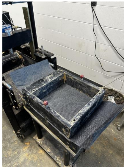
Figure 13. Wicking geotextile clamped to the shear box
