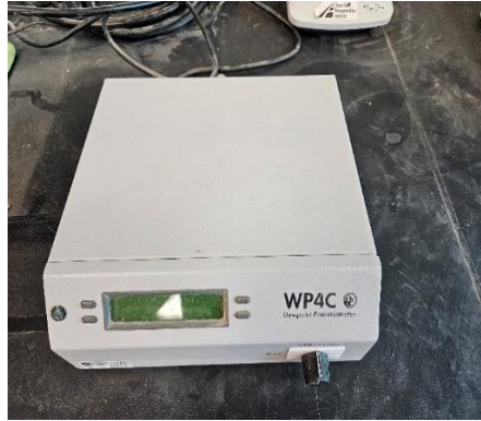
Figure 7. Potentiometer used in SWCC test
