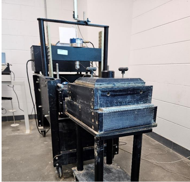
Figure 10. Large Scale Direct Shear Test Setup
