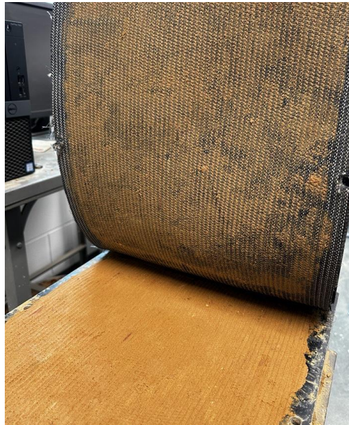
Figure 23. Grooves from geotextile in soil after test
