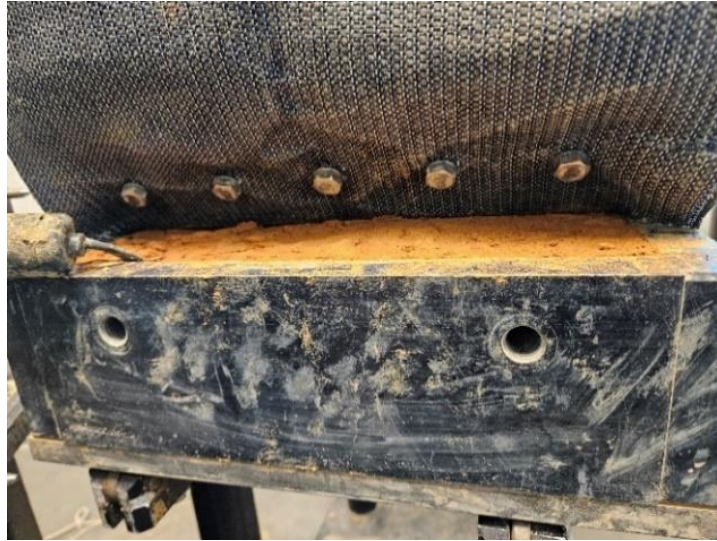
Figure 12. Geotextile fastened to top shear box
