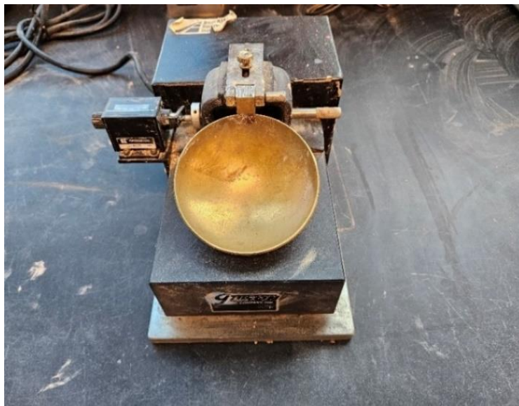
Figure 2. Casagrande device used for the liquid limit test
