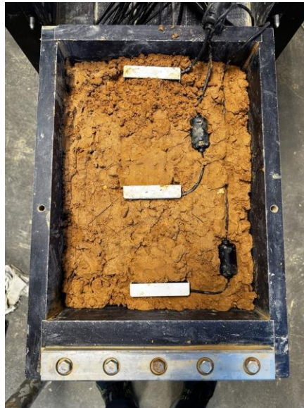
Figure 11. Moisture sensors placed in the bottom box
