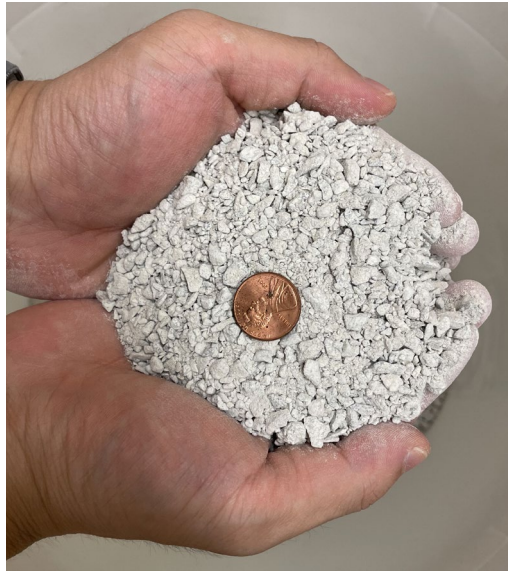
Figure 55. Photo. Close-up view of aggregate QB depicting sand-sized gradation.
