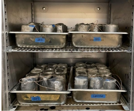
Figure 22. Photo. Cement-stabilized cylindrical QB specimens cured in the oven.
