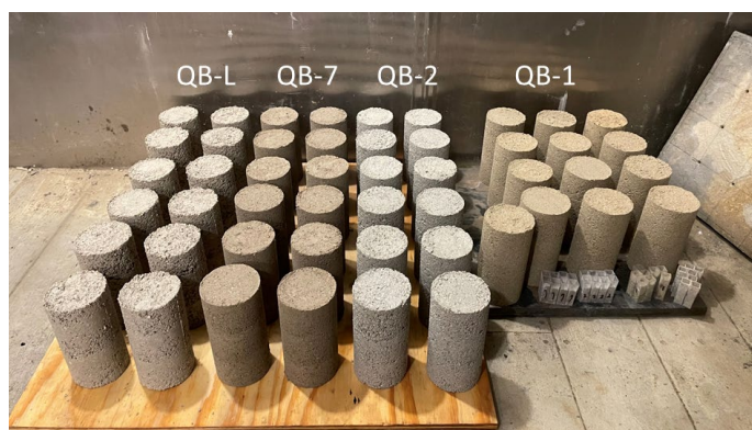
Figure 15. Photo. Cylindrical cement-stabilized QB specimens cured in a moisture room.
