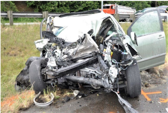
Figure 8. Front-plane damage, 2008 Toyota Sienna (police photo)
