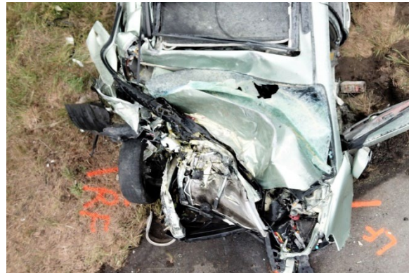
Figure 9. Front-plane damage, top view, 2008 Toyota Sienna (police photo)
