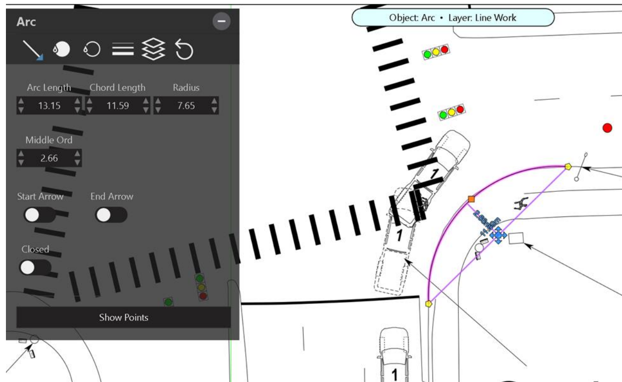
Figure 33. Example of Radius of Curvature, Vehicle Turning Right at Intersection
