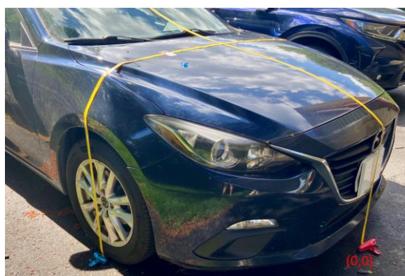
Figure 2. Example Bumper Height Measurement
