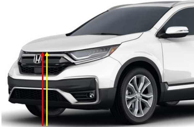
Figure 6. Front/Top Transition Point Equal to the Forward Hood Opening Height.
