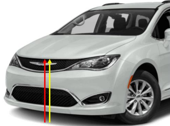
Figure 6. Front/Top Transition Point Equal to the Forward Hood Opening Height.
