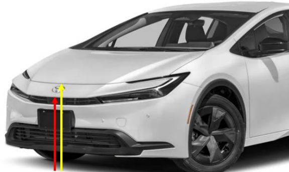
Figure 7. Front/Top Transition Point Below the Forward Hood Opening Height.
