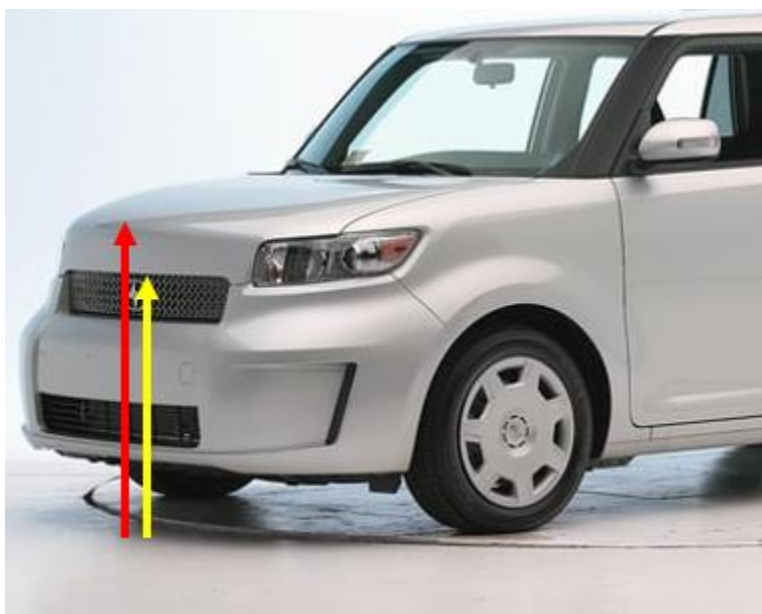
Figure 5. Front/Top Transition Point Above the Forward Hood Opening Height.
