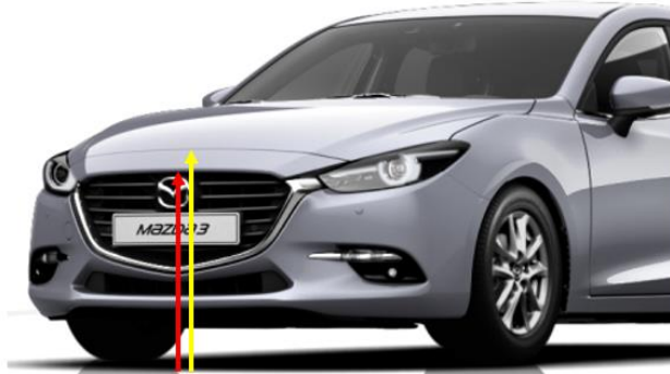
Figure 7. Front/Top Transition Point Below the Forward Hood Opening Height.
