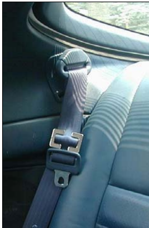
Figure 169. Locking clip correctly positioned on belt webbing
