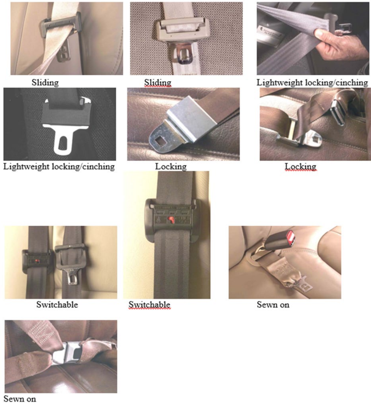
Figure 214. Examples of latch types on seat belts
