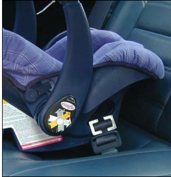
Figure 168. Locking clip correctly positioned on belt webbing near sliding latch plate
