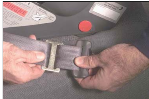
Figure 211. Locking clip affixed to belt webbing no more than 1 inch above latch plate
