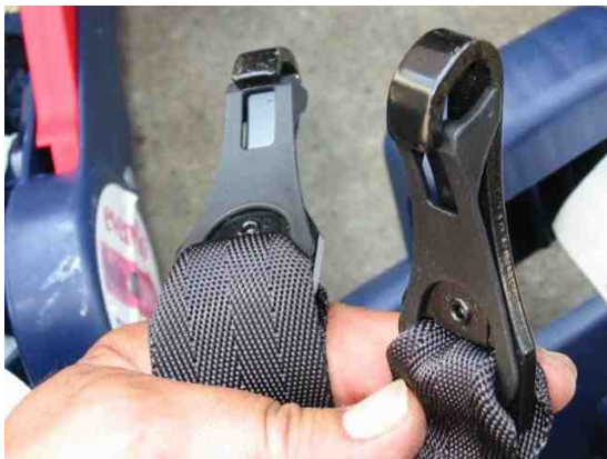
Figure 207. LATCH lower anchor attachments
