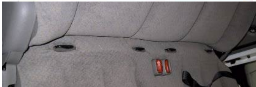
Figure 172. Example of lower child seat anchorage points
