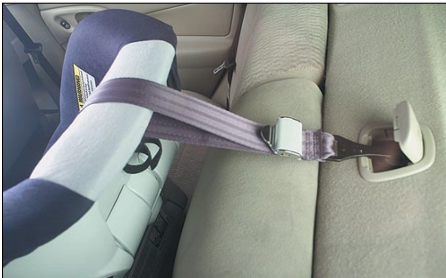
Figure 206. LATCH system top tether attached
