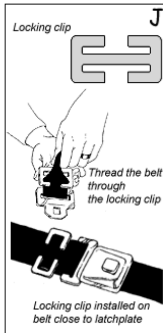
Figure 166. General instructions on how to position locking clip
