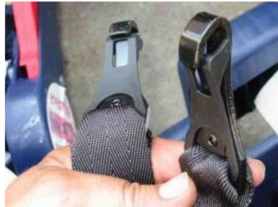
Figure 164. LATCH lower anchor attachments
