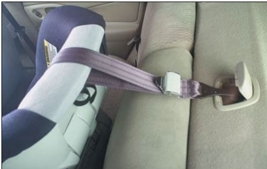
Figure 162. LATCH system top tether attached
