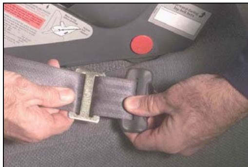
Figure 167. Locking clip affixed to belt webbing no more than 1 inch above latch plate
