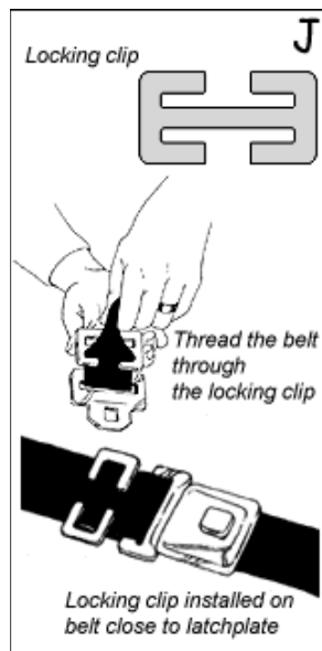
Figure 210. General instructions on how to position locking clip
