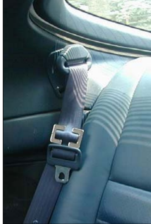
Figure 212. Locking clip correctly positioned on belt webbing near sliding latch plate
