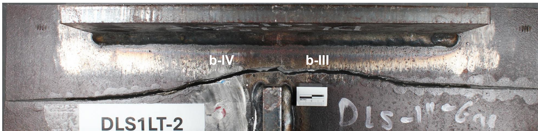
Figure 96. Photograph. DLS1LT-2: top view of fractured specimen.
