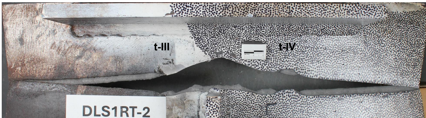
Figure 100. Photograph. DLS1RT-2: top view of fractured specimen.
