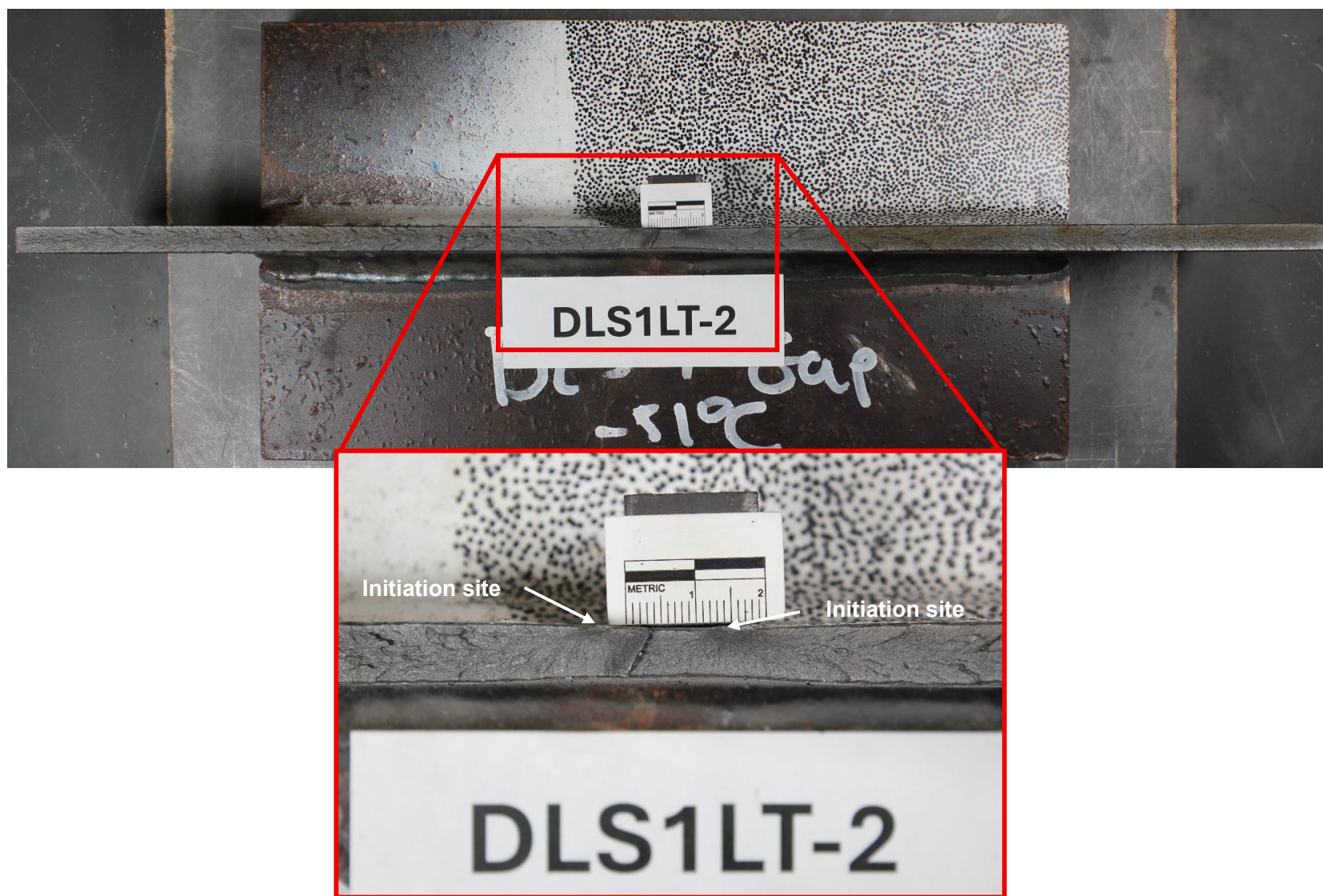
Figure 98. Photograph. DLS1LT-2: transverse-stiffener side of fracture.
