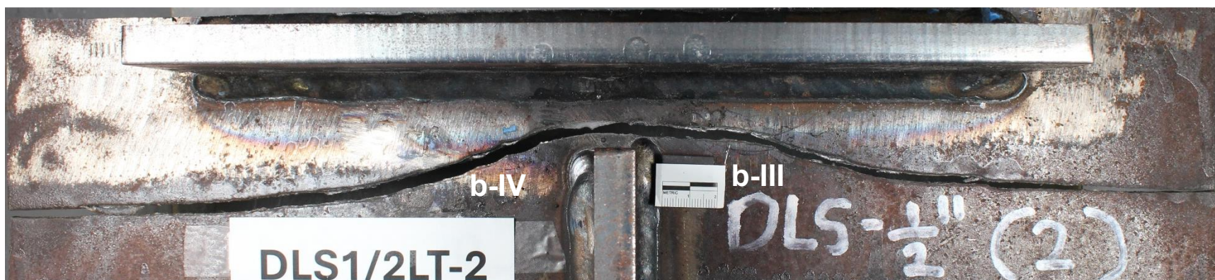
Figure 91. Photograph. DLS1/2LT-2: bottom view of fractured specimen.
