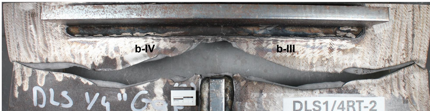
Figure 81. Photograph. DLS1/4RT-2: top view of fractured specimen.
