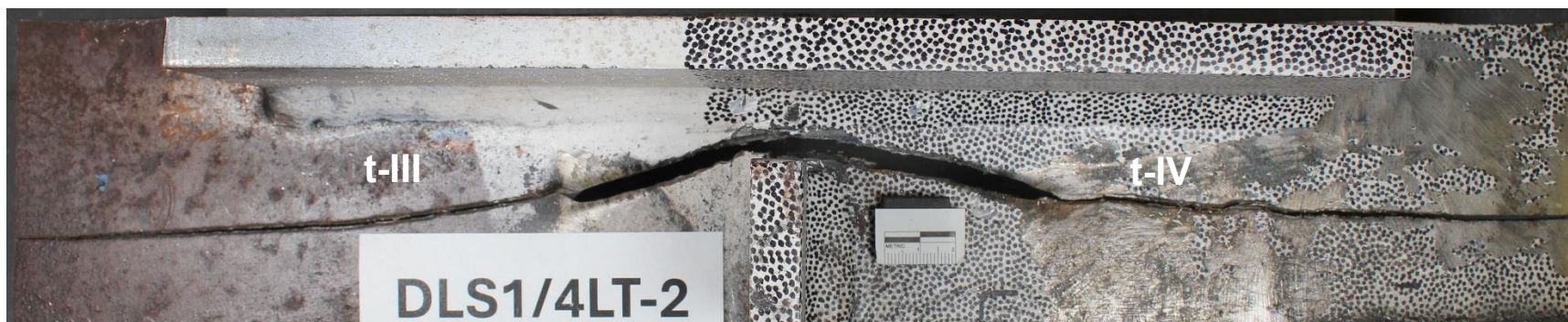
Figure 76. Photograph. DLS1/4LT-2: top view of fractured specimen.
