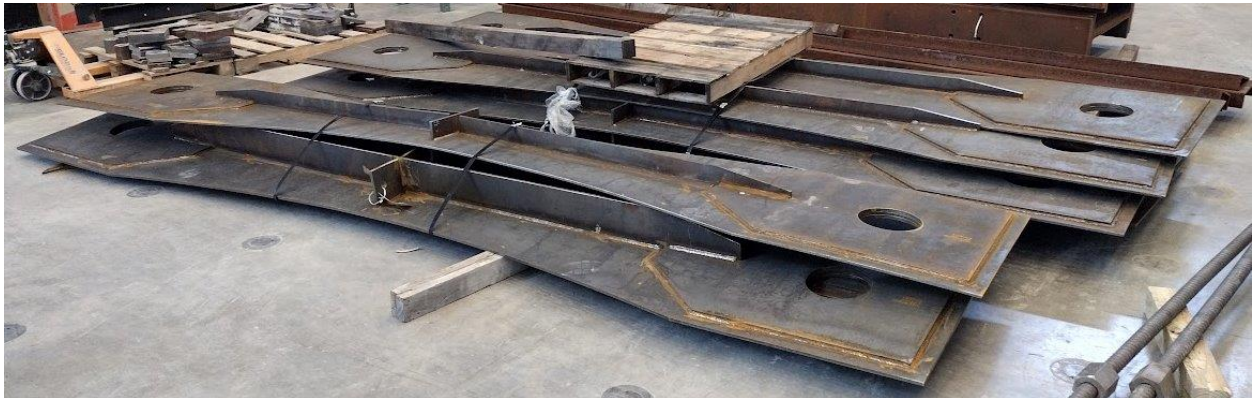
Figure 53. Photograph. Dog-bone specimens in the KU West Campus Structural Testing Laboratory.
