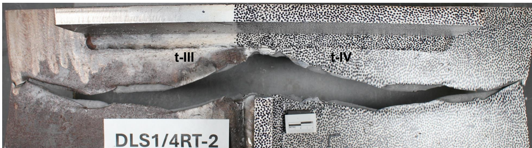
Figure 80. Photograph. DLS1/4RT-2: top view of fractured specimen.
