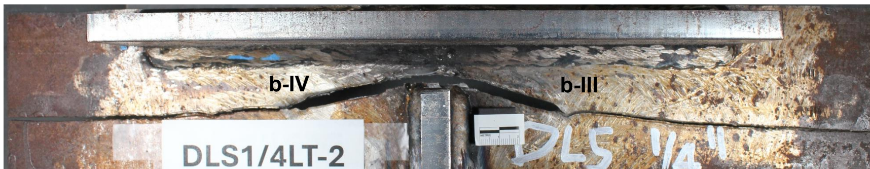
Figure 77. Photograph. DLS1/4LT-2: bottom view of fractured specimen.
