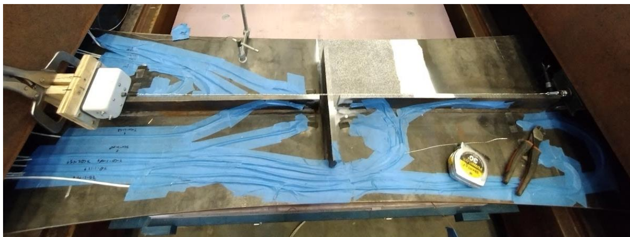
Figure 51. Photograph. String potentiometer installed on a test specimen.
