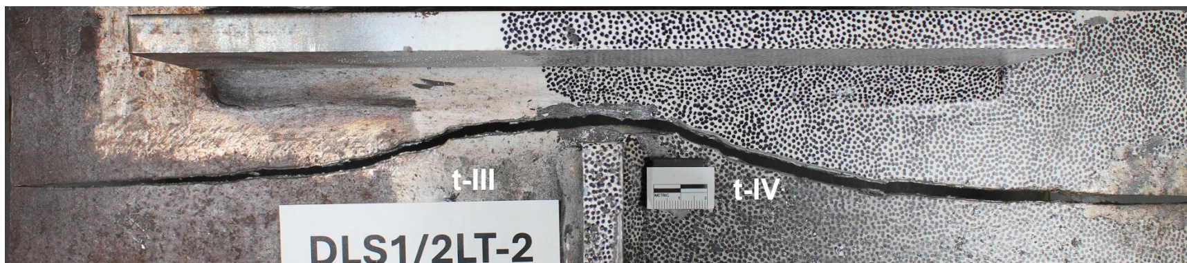
Figure 90. Photograph. DLS1/2LT-2: top view of fractured specimen.
