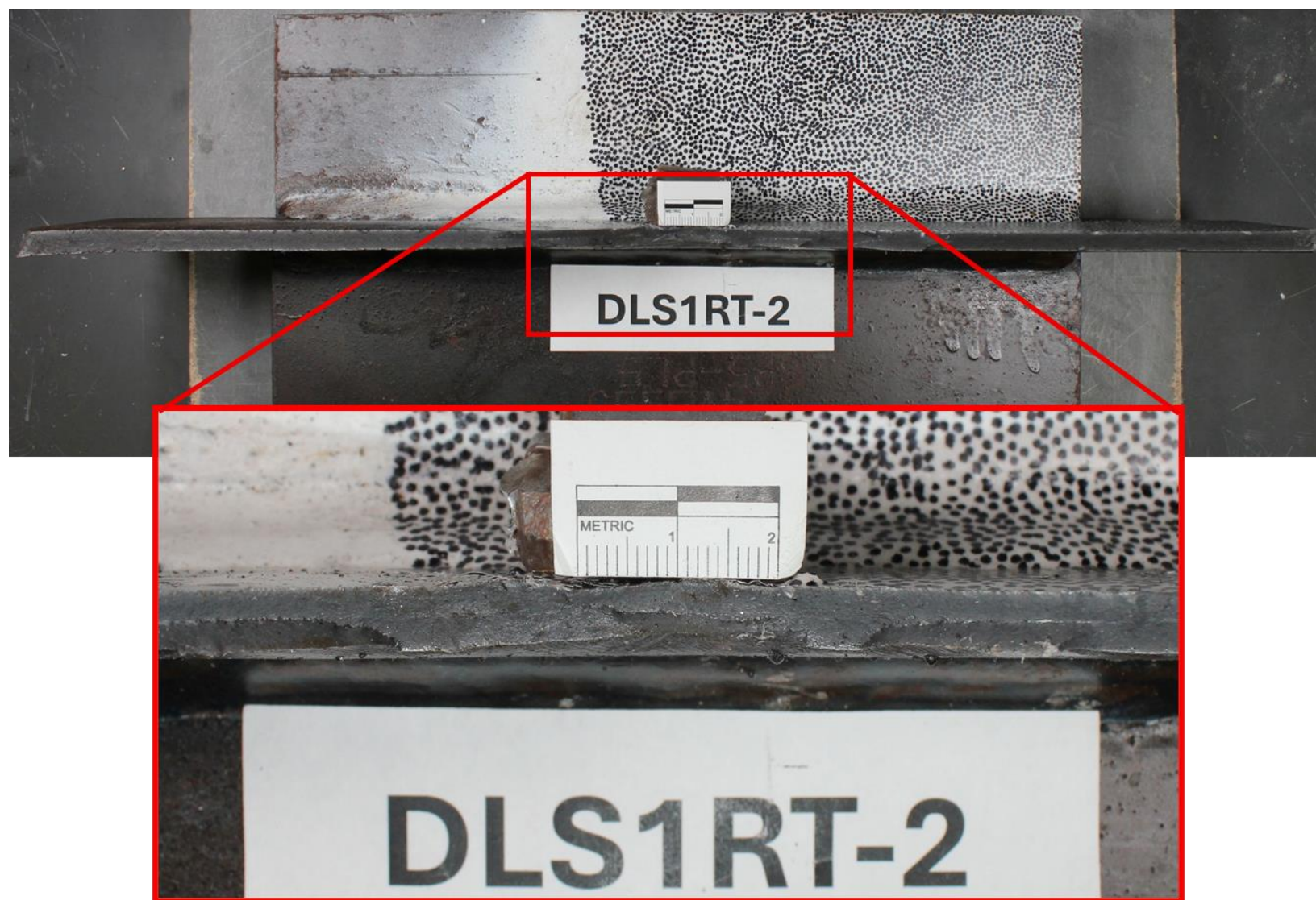
Figure 102. Photograph. DLS1RT-2: transverse-stiffener side of fracture.
