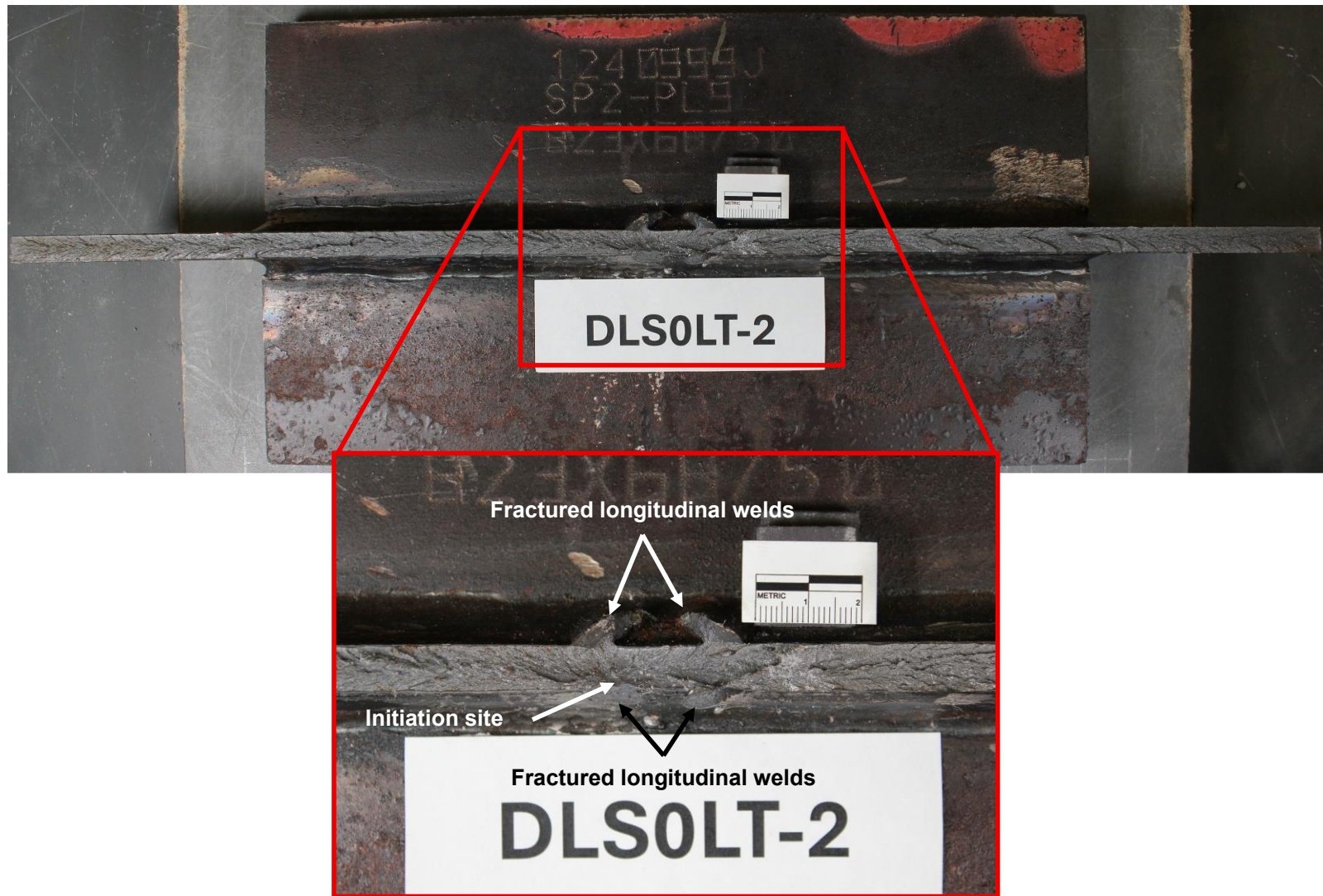
Figure 71. Photograph. DLS0LT-2: transverse-stiffener side of fracture.
