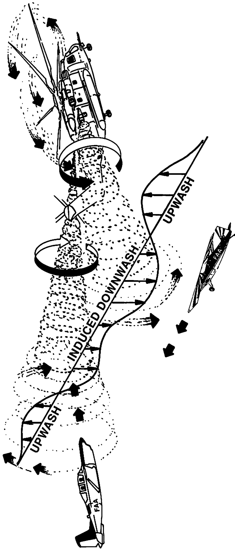
Figure 1. Vortex probing techniques.
