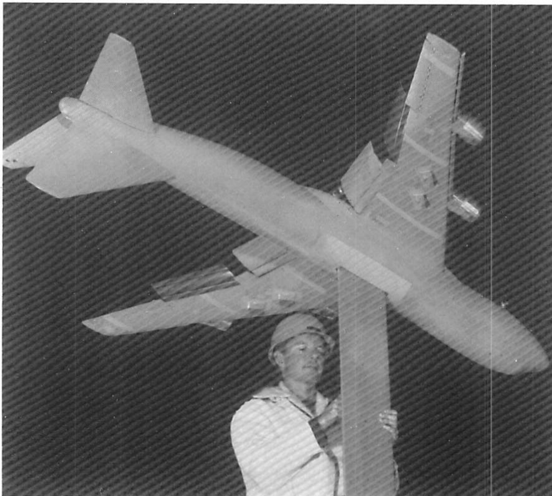
b. Closeup view of model of B-747 mounted upside down on support strut with two circular-arc fins mounted midway out on each wing.
