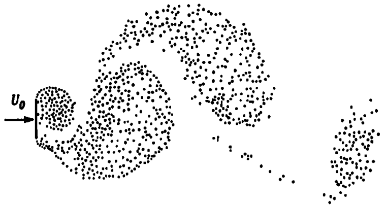
Calculated vortex wake behind a flat plate in the case of asymmetric flow (Kármán vortex street).
