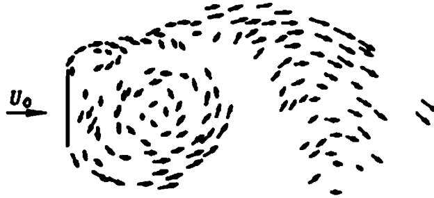
Asymmetric separated flow past a flat plate for Re = \infty, \alpha = 90^\circ : (a) towing tank tests, (b) calculated.
