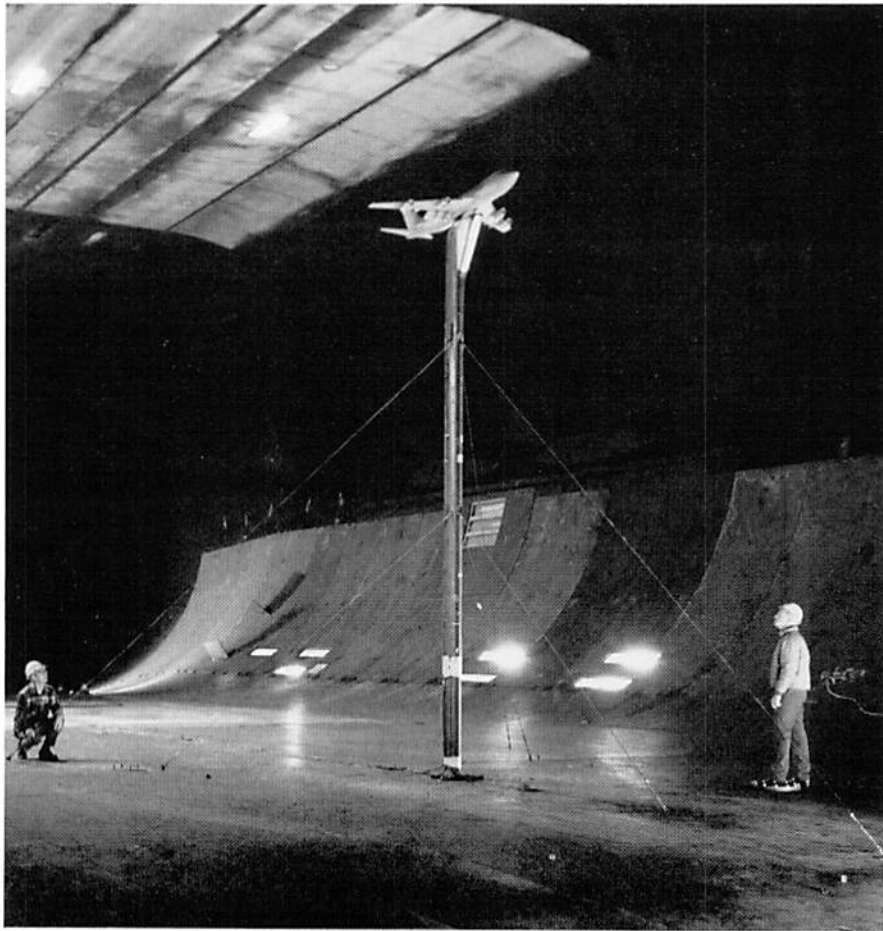
Figure 10. Strut configuration used to support B-747 wake-vortex generating model during first entry into 40- x 80-foot wind tunnel.
