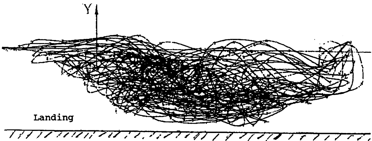
Figure 11. Helicopter wake at landing.
