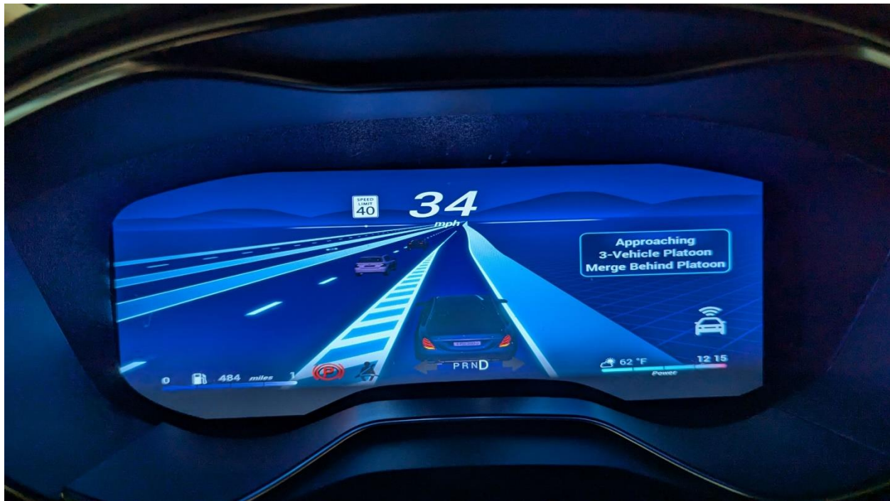
Figure 1. Photo. Text displayed on the instrument cluster by a V2V CDA alert indicating a three-vehicle platoon is approaching.
