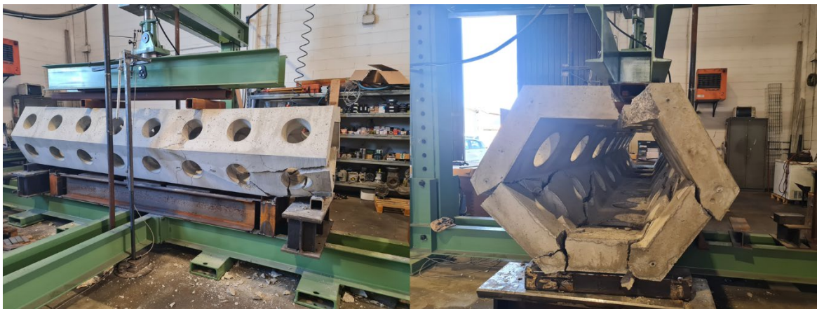
Figure 38: Damaged representation of specimen C2
