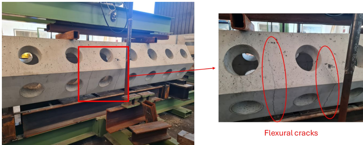
Figure 17: Flexural crack formation at specimen A2
