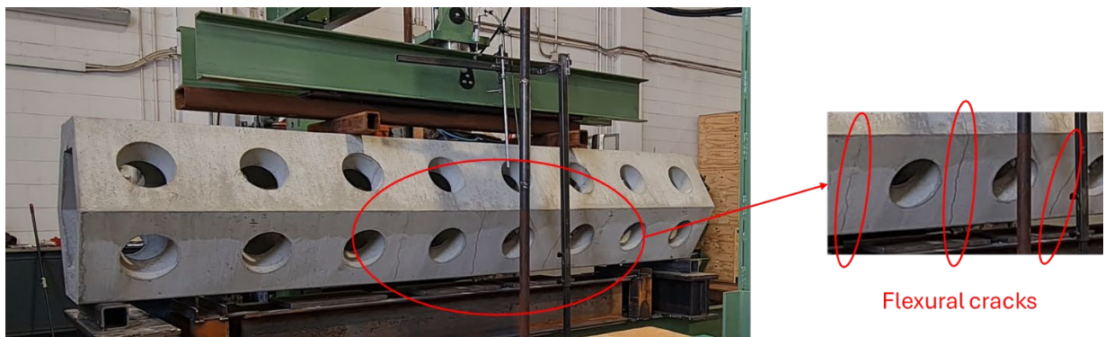
Figure 22: Flexural crack formation at specimen B1
