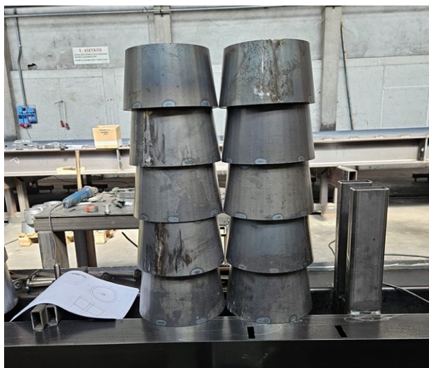
Figure 2: Stack of steel cones for perforating SEAHIVE® prestressed modules (Patent pending filed by SIGMAc s.r.l., Vicenza, Italy).
