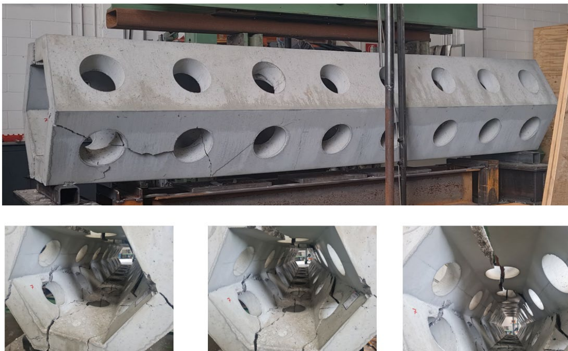
Figure 13: Damaged representation of specimen A1
