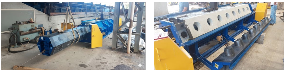
Figure 8: Demolding of SEAHIVE® module with lifting equipment (Patent pending filed by SIGMAc s.r.l., Vicenza, Italy)
