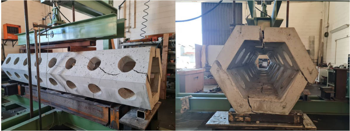
Figure 18: Damaged representation of specimen A2
