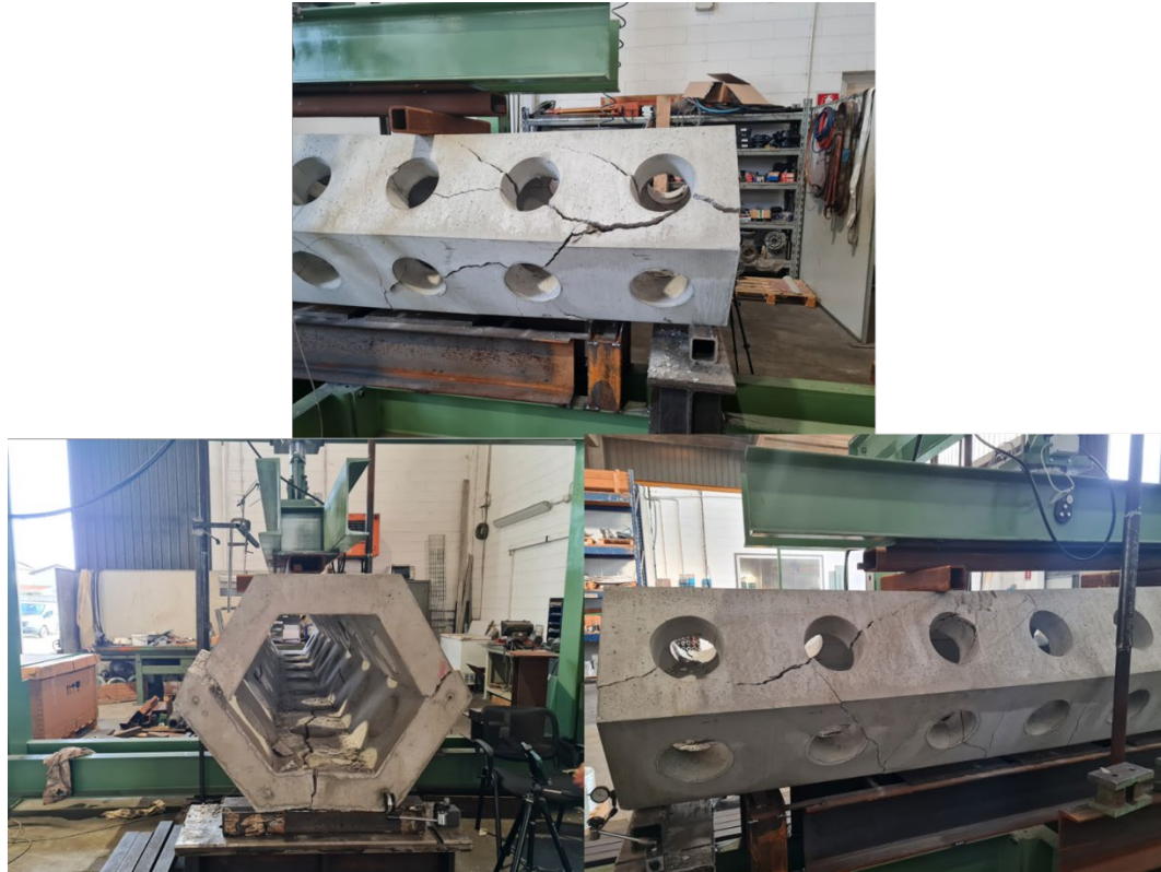
Figure 23: Damaged representation of specimen B1
