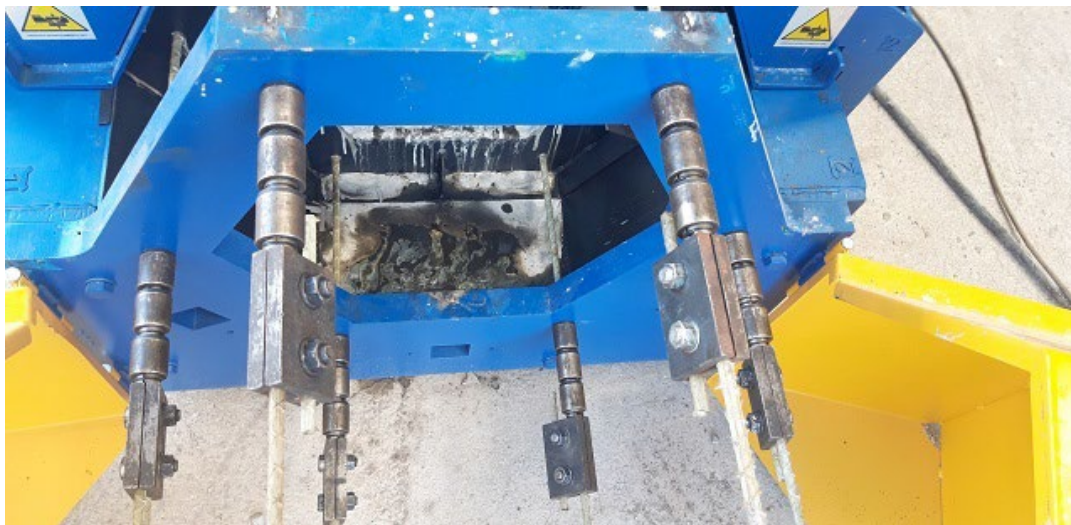
Figure 5: Prestressing of GFRP bars in SEAHIVE® module fabrication (Patent pending filed by SIGMAc s.r.l., Vicenza, Italy).
