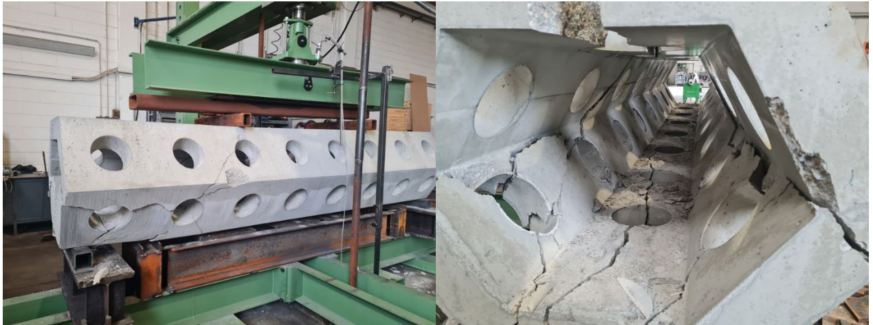
Figure 33: Damaged representation of specimen C1
