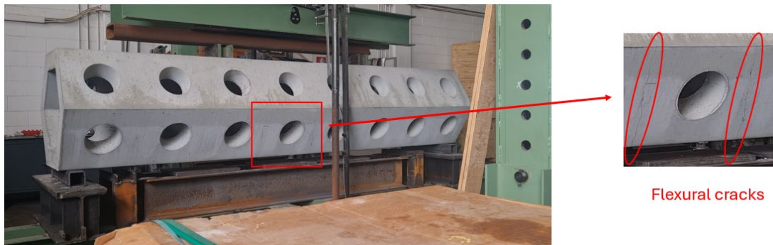
Figure 12: Flexural crack formation at specimen A1
