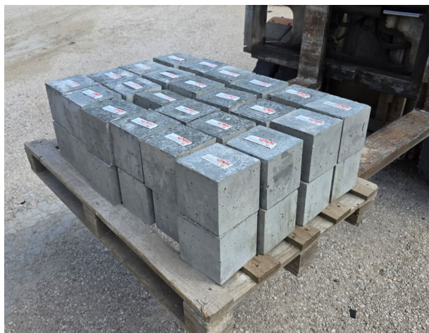
Figure 7: Fabrication of cubic samples during SEAHIVE® specimens casting.
