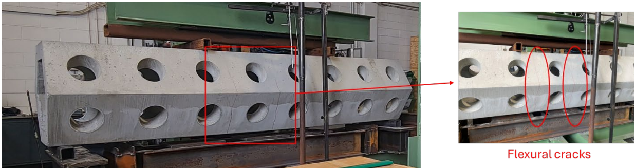
Figure 32: Flexural crack formation at specimen C1
