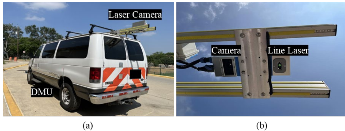
Figure 4. Pavement survey vehicle: (a) Position of distance measurement unit (DMU) and line laser sensor camera; (b) Line laser and camera.
