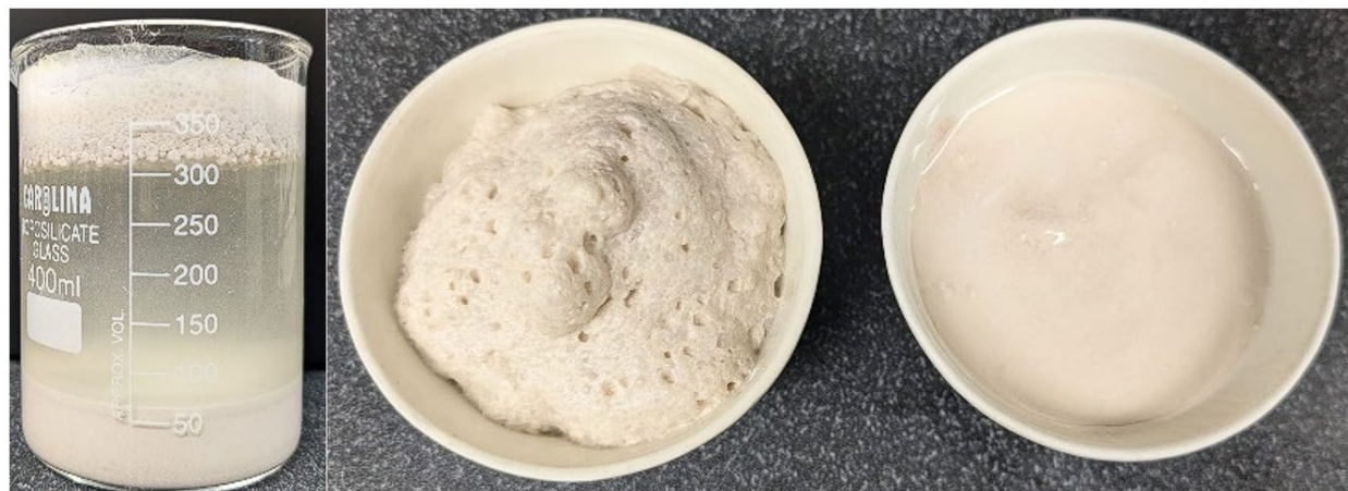
Figure 5: Stratification of eggshell powder in water, with sample collected from the water surface (left) and bottom of vessel (right).
