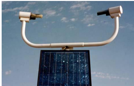
Figure 5. Visibility sensor utilized by the Idaho DOT (Koeberlain, Christensen, and Dwight, Idaho DOT)
