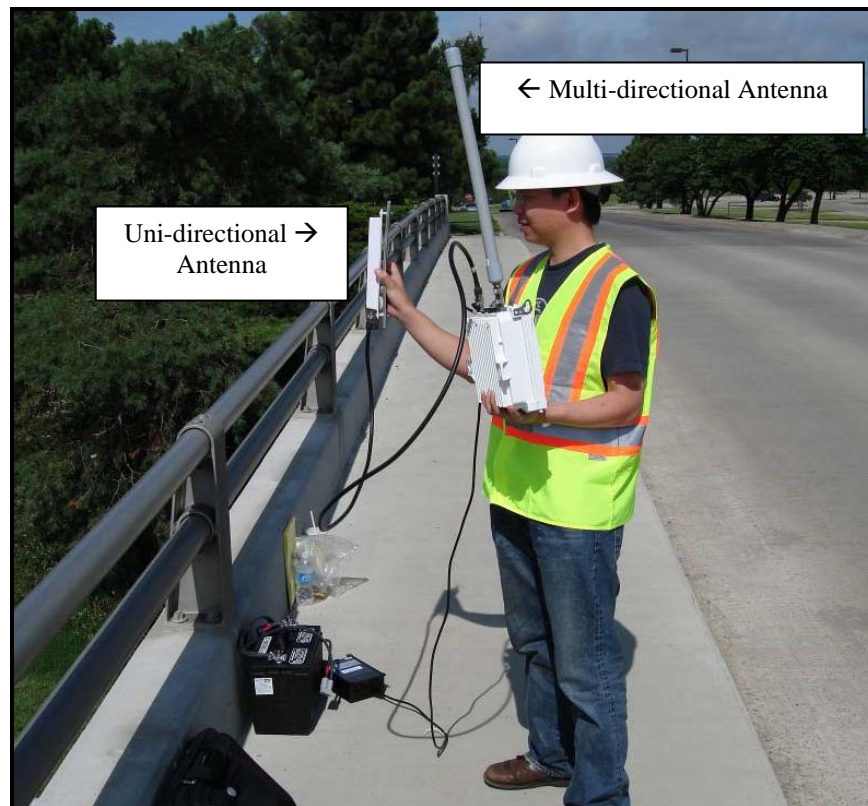
FIGURE 2 Mesh Router with Multi-directional and Uni-directional Antenna
