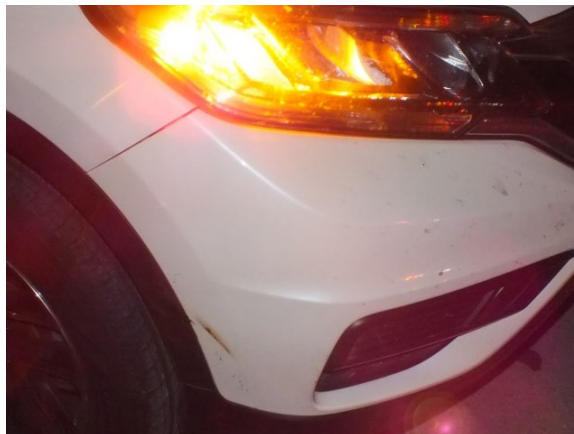
Figure 6. Right plane damage, the 2016 Honda CR-V (police photo)
