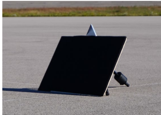
Figure 2. Example of trihedral corner reflector affixed to tripod masked with reticulate foam
