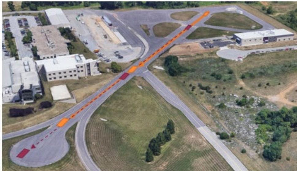
Figure 37. SV and TV positions for lane slalom and low-speed range sweep
