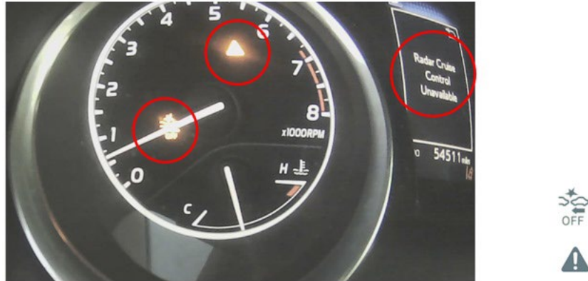
Figure 75. ADAS sensor self-diagnostics reporting a system error for Vehicle 1
