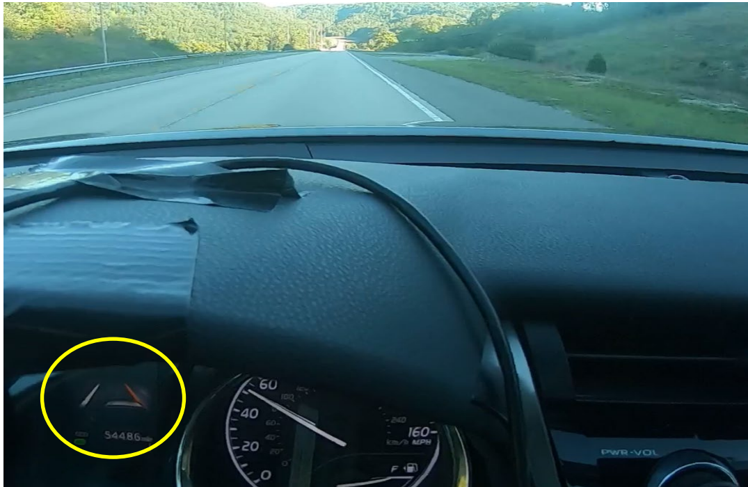
Figure 71. An example of the system correctly detecting the left lane line (see bold left lane line in yellow circle) and issuing a right LDW (see red lane line)
