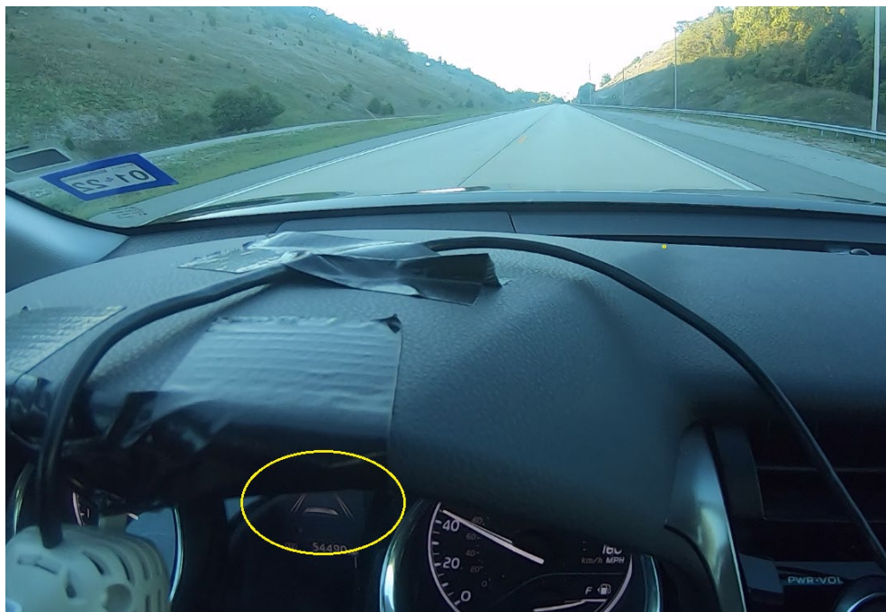
Figure 72. Example of the system not detecting any lane lines and did not issue a left LDW (two errors) and did not detect the right lane line (one error)
