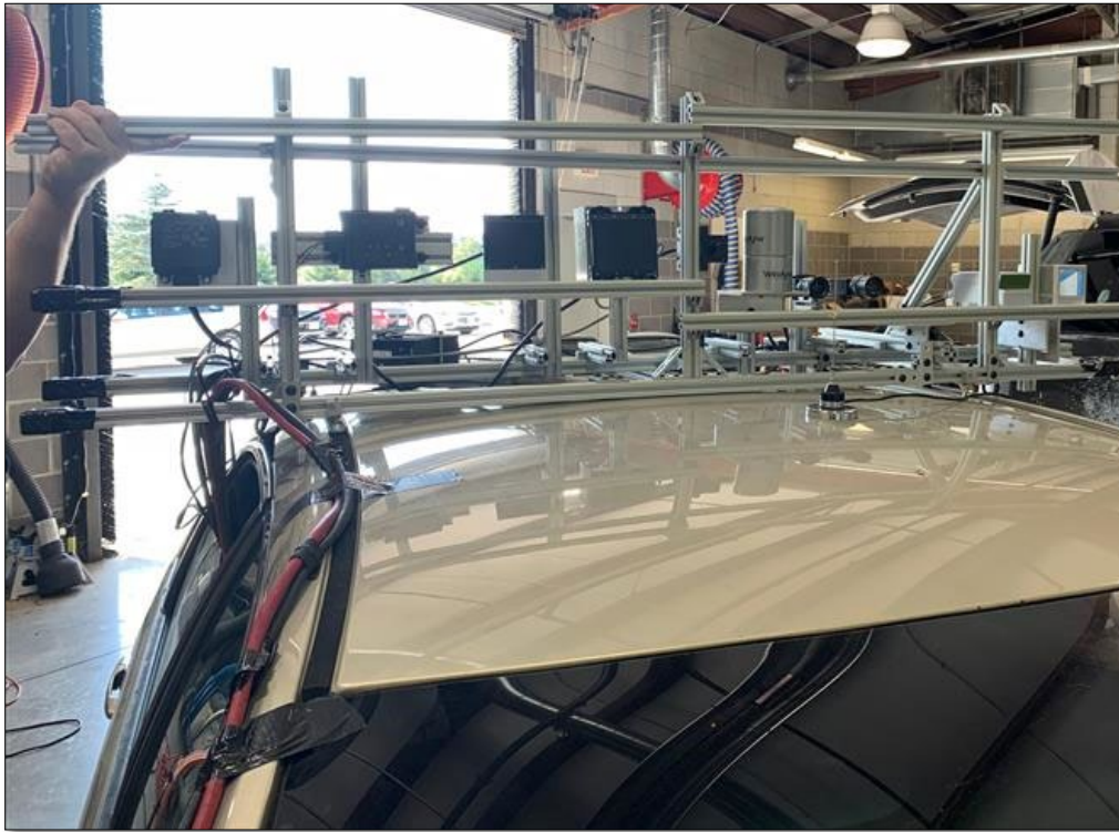
Figure 36. SV with sensor frame and sensors
