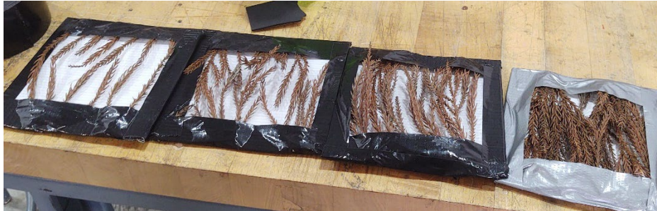
Figure 81. Biological material degradations from lightest to heaviest (left to right)
