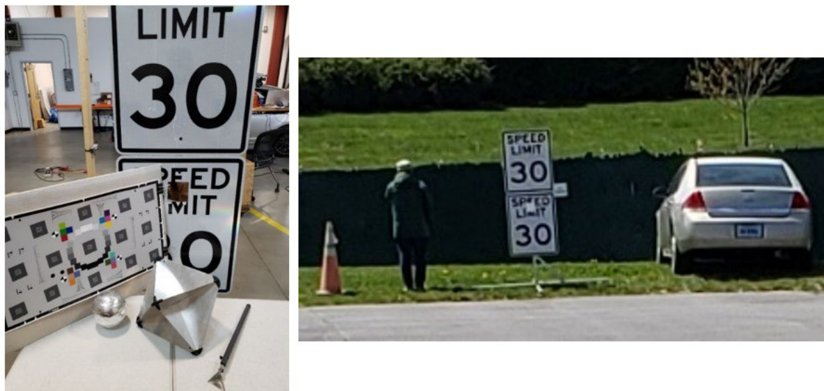
Figure 21. Targets used to compare the effect of base materials and degradations
