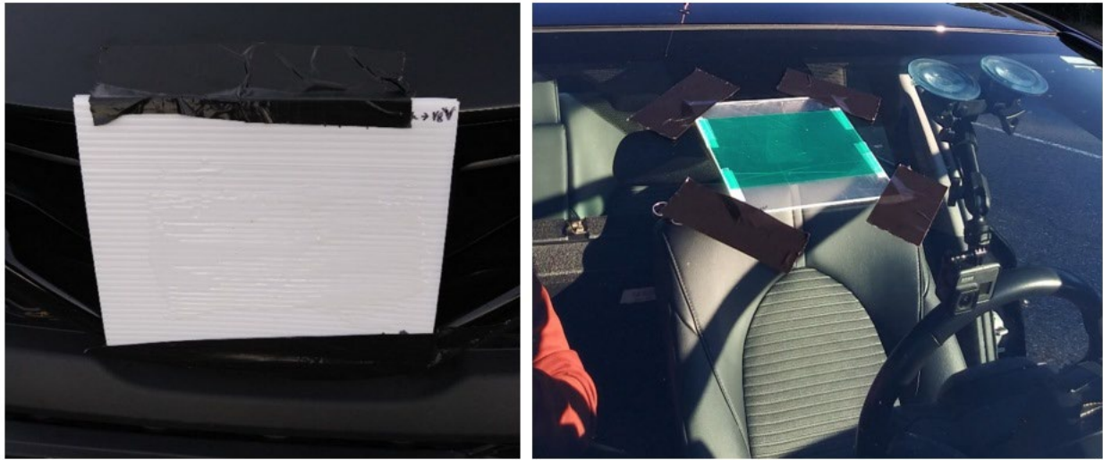
Figure 70. Radar and optical degradation placement
