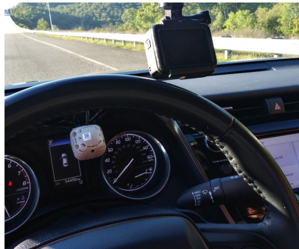
Figure 68. Camera placement for the instrument cluster
