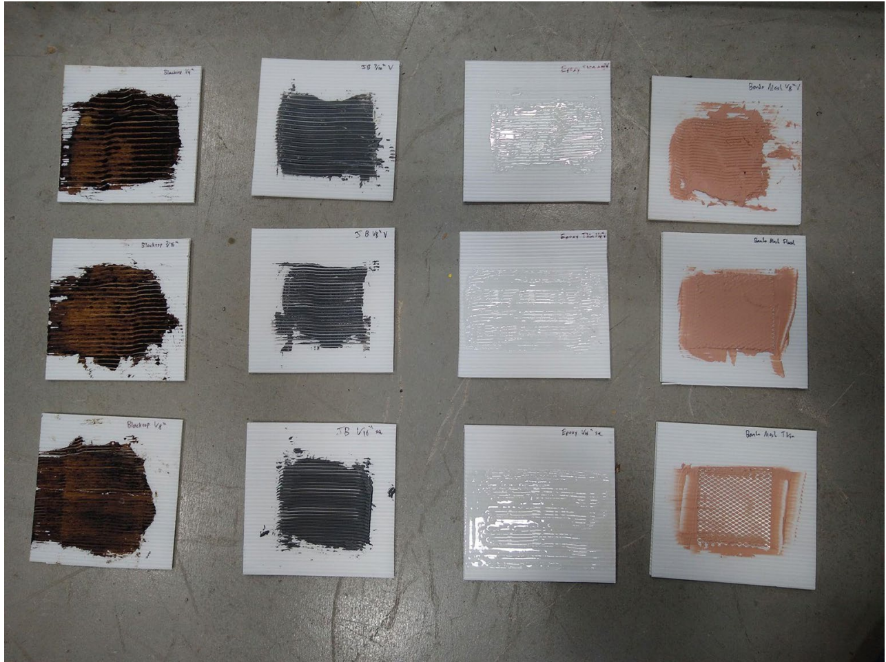
Figure 34. Polyethylene specimens prepared for radar testing
