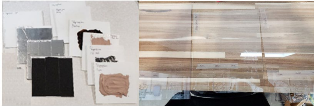
Figure 22. Samples of simulated degradations (left: bumper degradations; right: optical degradations)
