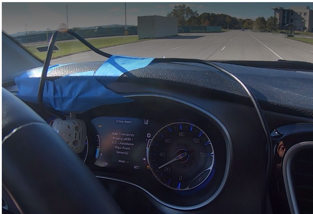
Figure 76. ADAS sensor self-diagnostics of Vehicle 3
