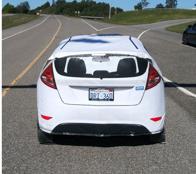
Figure 69. Deployed GVT for FCW and AEB testing
