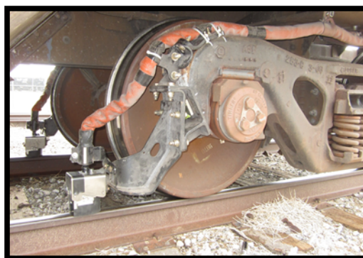
Fig 5: Friction Modifier Spray Application Nozzles
