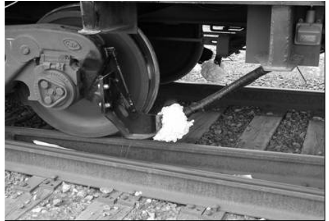
Figure 5: Ore Car TOR Nozzle Mounting Details
