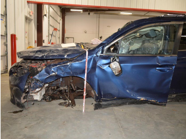
Figure 12. Damage to the left front of the Subaru from Event 1
