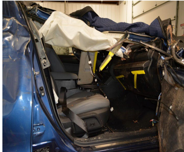
Figure 21. View of the intrusion and deployment damage to the front passenger's seat and right A-pillar area
