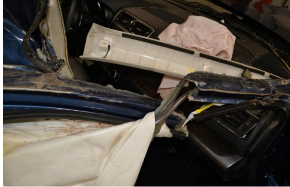
Figure 17. Right A-pillar separation during Event 5
