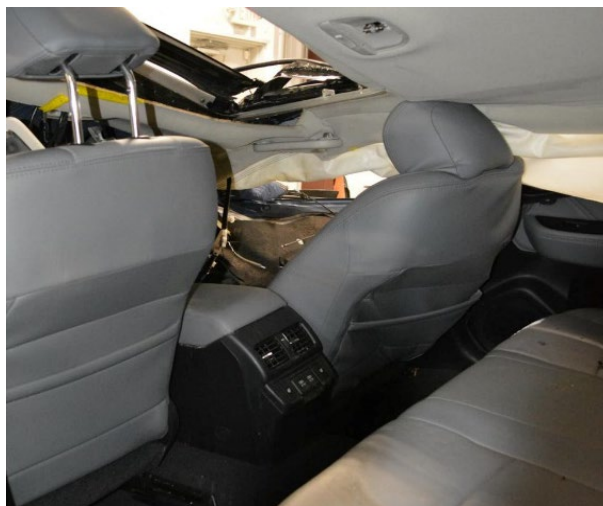
Figure 22. View of the front row intrusion from the second row and B-pillar intrusion
