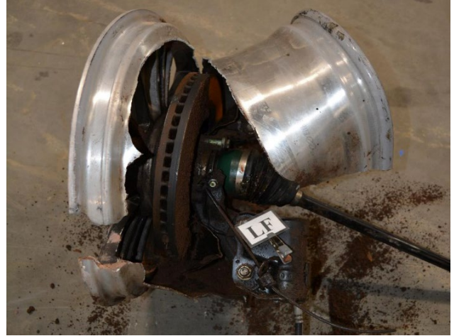
Figure 13. Damage to the center left front wheel assembly
