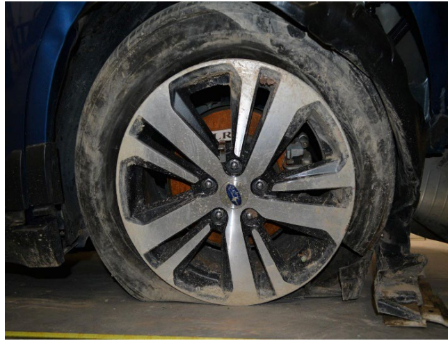
Figure 14. Damage to the left rear tires from Events 2 and 3
