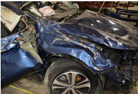
Figure 15. Damage along the right front panel from Event 5
