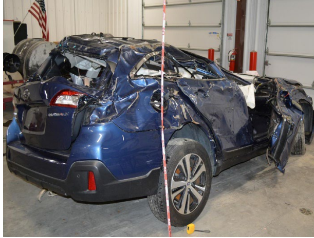
Figure 19. Damage to the back of the Subaru from Event 7
