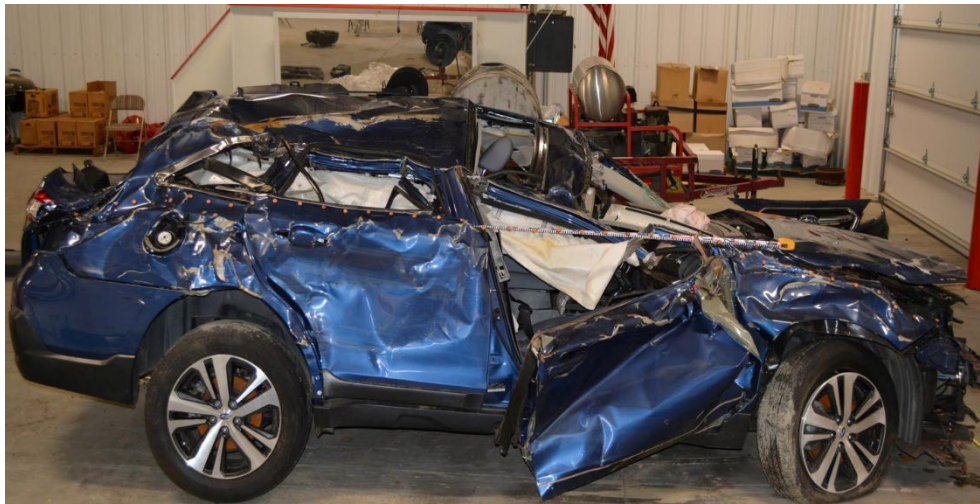
Figure 18. Overlapping damage to the right side from Events 4-6
