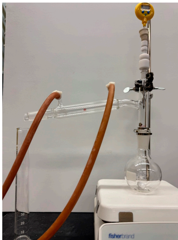
Figure 3. Apparatus used for distillations.
