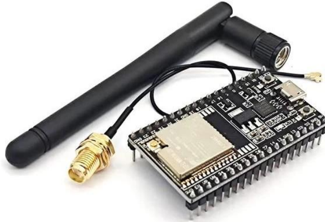
Figure 7. Photo. ESP32 microcontroller with on-board antenna.
