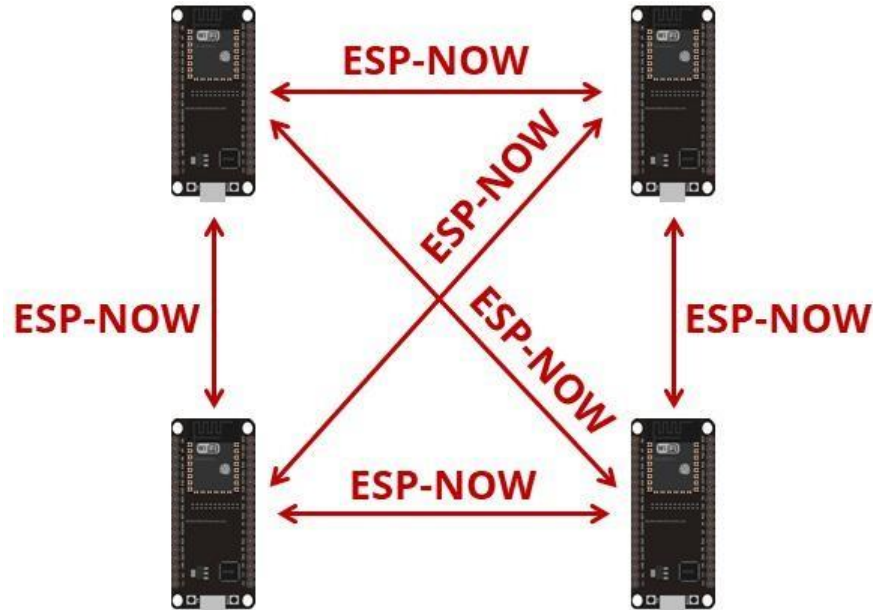
Figure 8. Diagram. ESP32 ESP-NOW communication.
