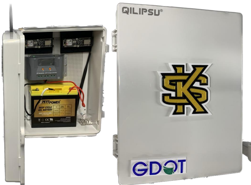
Figure 12. Photos. Receiver assembly and enclosure.
