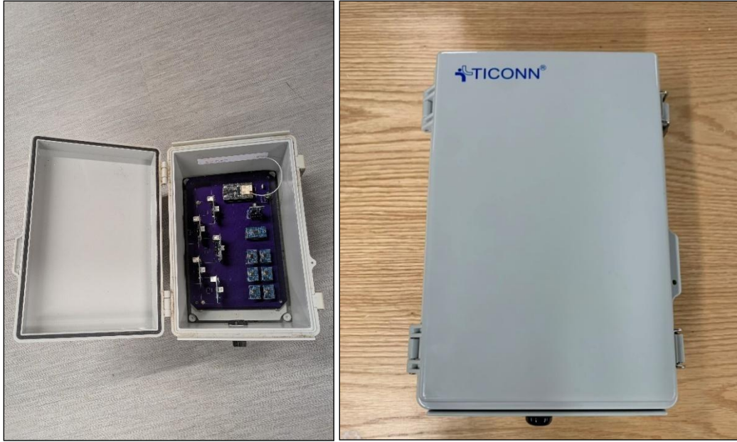
Figure 13. Photos. Transmitter assembly and enclosure.
