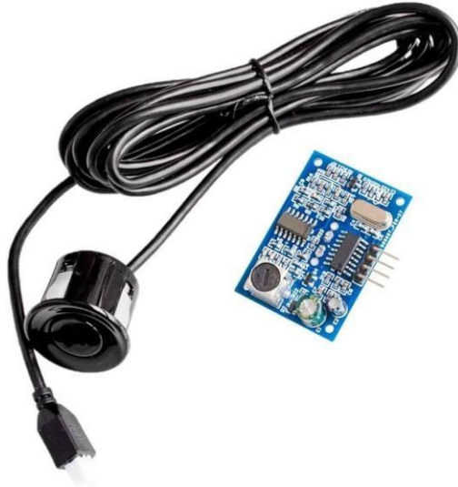
Figure 6. Photo. JSN-SR04T sonar transmitter and receiver.
