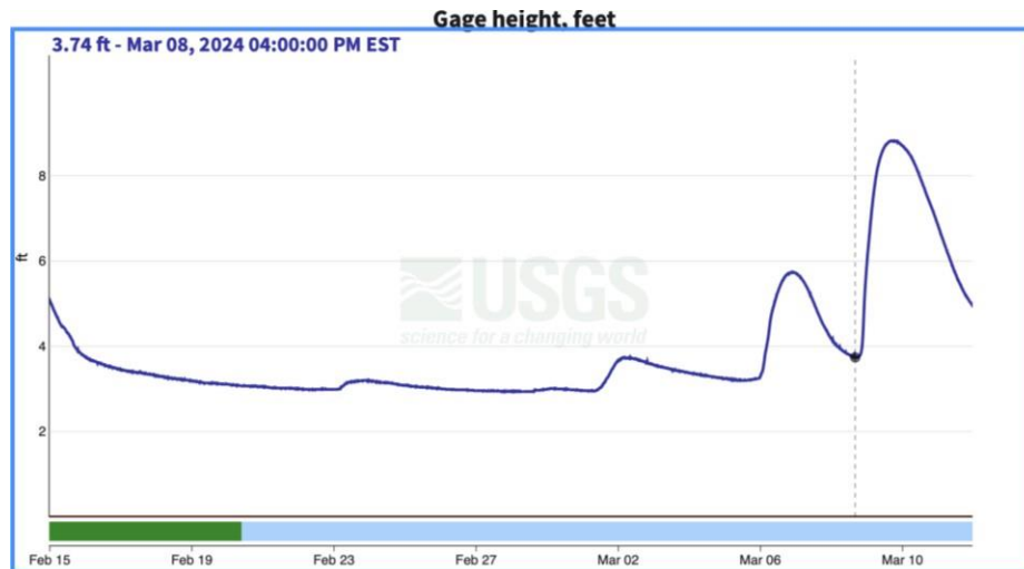
Figure 61. Graph. Flooding hydrograph, March 8, 2024.
