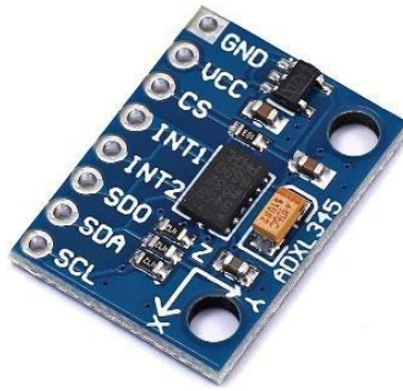
Figure 5. Photo. ADXL345 accelerometer.
