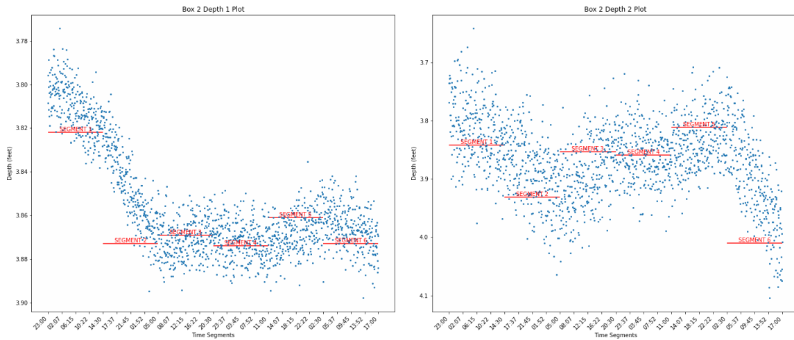
Figure 65. Plots. Scour depth output plots, Depths 1 and 2, Bridge 2, Flood 3.
