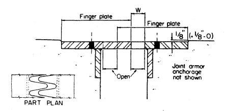
Figure 7-8 Cantilever Finger Plate Joint
