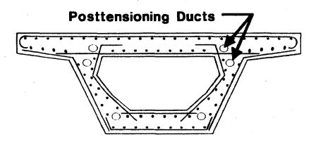
Figure 9-34 Longitudinal Reinforcement in a Concrete Box Girder
