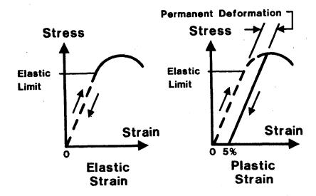
Figure 3-6 Stress-Strain Diagram
