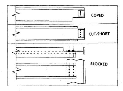
Figure 18-8 Cut Short, Coped, and Blocked Beam Flanges
