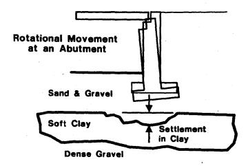
Figure 12-7 Rotational Movement of an Abutment
