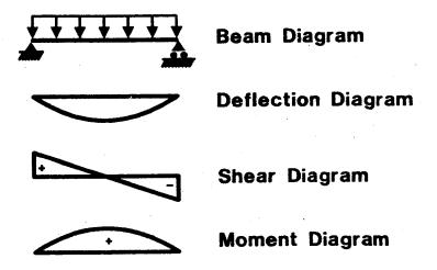
Figure 3-14 Simple Span
