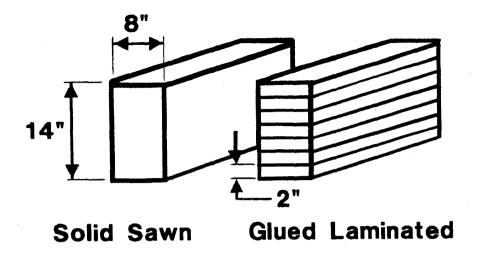
Figure 6-11 Timber Beams
