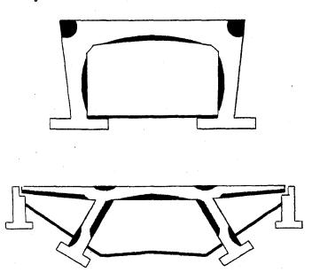
Figure 9-22 Tension Areas (Shown in Black) in Rigid Frames Due to Gravity Loads
