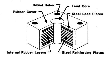
Figure 11-11 Lead Core Isolation Bearing
