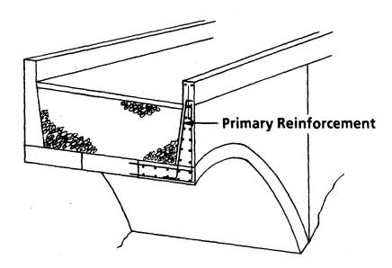
Figure 9-18 Reinforcement in a Closed Spandrel Arch
