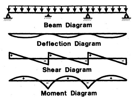
Figure 3-15 Continuous Span
