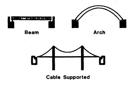
Figure 2-1 Three Basic Bridge Types (Source: 18)
