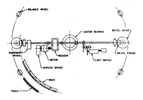
Figure 20-5 Layout of Center Bearing Type Swing Span with Machinery on the Span
