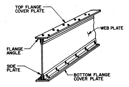
Figure 6-17 Riveted I-Beam
