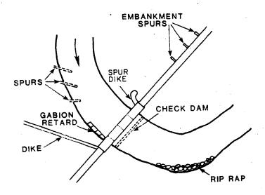
Figure 13-3 Placement of Flow Control Structures (Source: 85)
