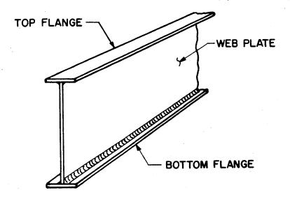
Figure 6-19 Welded I-Beam
