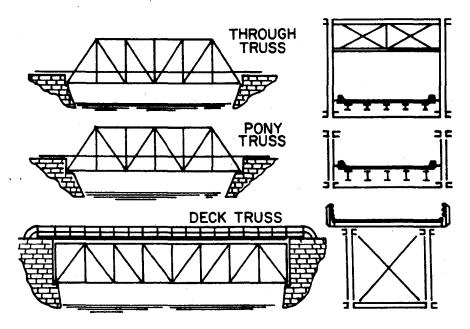
Figure 10-10 Comparison of Through, Pony, and Deck Trusses
