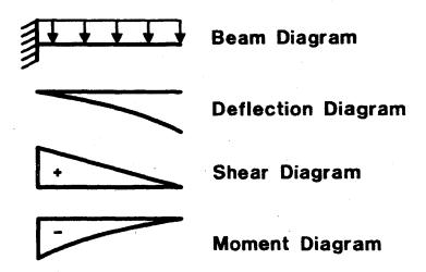
Figure 3-16 Cantilever Span
