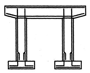
Figure 12-11 Primary Reinforcing Steel in Column Bents
