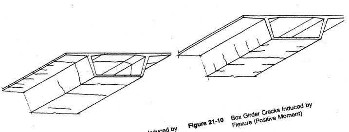
Box Girder Cracks Induced by Direct Tension Figure 21-9
