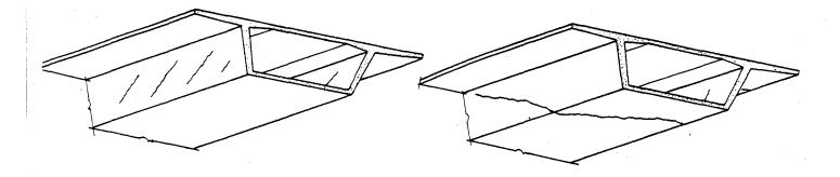
Figure 21-13 Box Girder Cracks Induced by Shear
