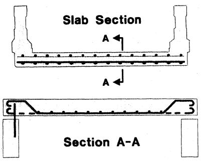
Figure 9-2 Steel Reinforcement in a Concrete Slab
