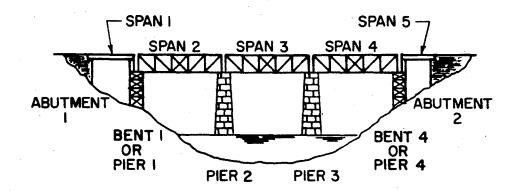
Figure 5-3 Sample Bridge Numbering Scheme
