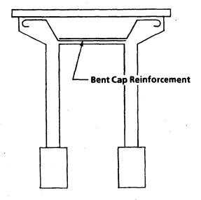
Figure 9-15 Spandrel Bent Cap Reinforcement
