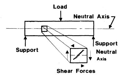
Figure 3-11 Shear Forces in a Member Element
