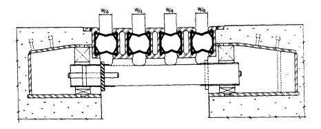
Figure 7-11 Modular Elastomeric Seal
