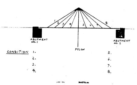
Figure 21-6 Form for Recording Defects in Cable System of a Cable-Stayed Bridge
