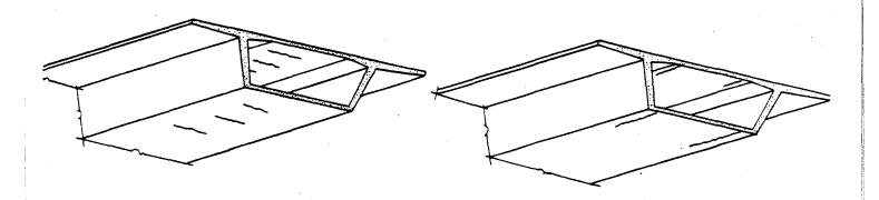
Figure 21-15 Thermally Induced Cracks in Box Girder Slab
