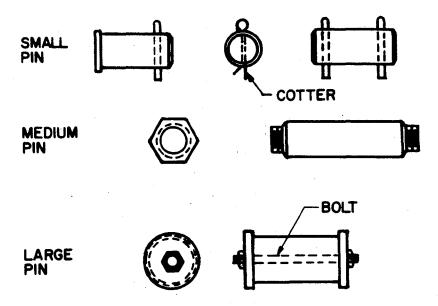
Figure 6-22 Sizes of Bridge Pins
