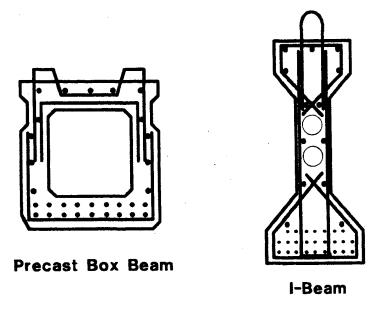
Figure 9-27 Reinforcement in Precast Box Beams and I-Beams
