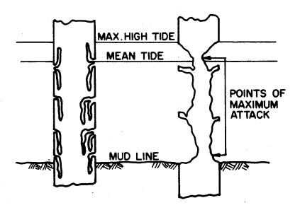
Figure 4-7 Drawing of Typical Borer Damage
