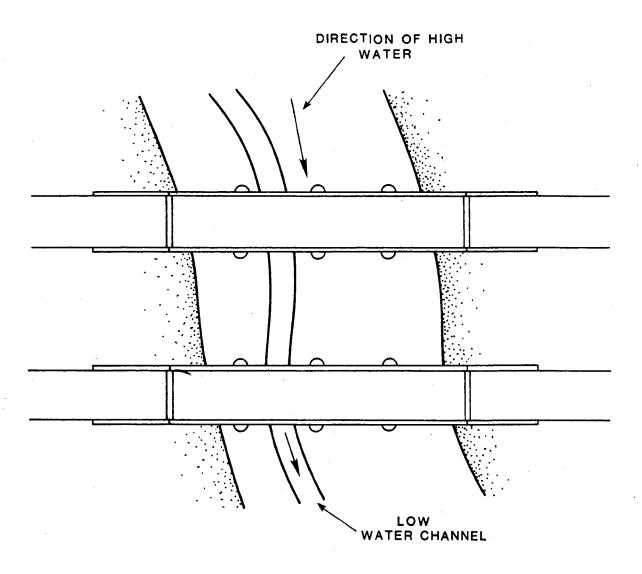
Figure 13-4 Typical Changes in Flow Alignment During High Water Causing Local Scour Around Piers
