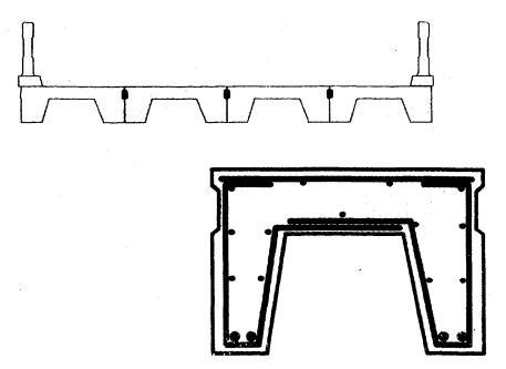
Figure 9-12 Channel Beam Cross Section
