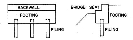
Figure 12-1 Common Abutment Types
