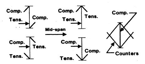
Figure 10-13 Prediction Method for Stresses in Truss Verticals
