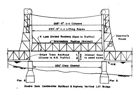
Figure 20-18 Outline of Double Deck Vertical Lift Bridge in Intermediate (Normal) Position to Provide Clearance for Small Boats Between Train Movements
