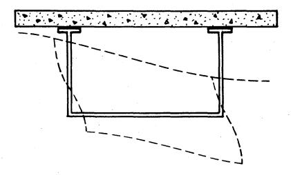
Figure 3-12 Torsional Distortion
