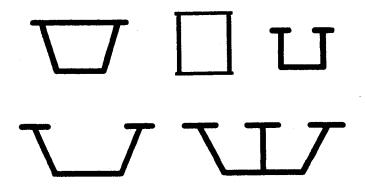
Figure 6-20 Welded Box Shapes
