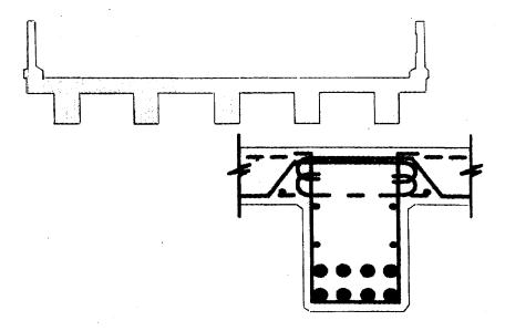
Figure 9-5 Steel Reinforcement in a Concrete Tee Beam
