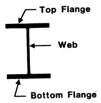
Figure 3-9 Girder Cross Section
