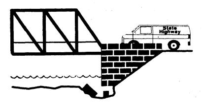
Figure 12-6 Abutment With Scour and Undermining
