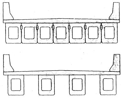
Figure 9-26 Applications of Prestressed Box Beams
