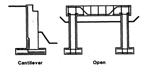
Figure 12-2 Primary Reinforcing Steel in Abutments
