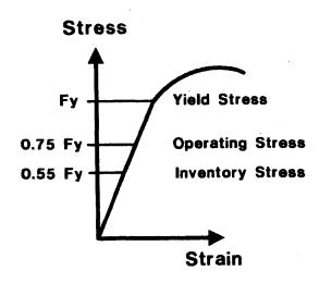
Figure 3-18 Bridge Load Capacity Rating Levels for Steel
