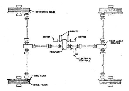
Figure 20-13 Vertical Lift Bridge Machinery is Located on Top of the Lift Truss Span, and the Operating Drums Rotate to Wind the Up-Haul (Lifting) Ropes as They Simultaneously Unwind the Down-Haul Ropes
