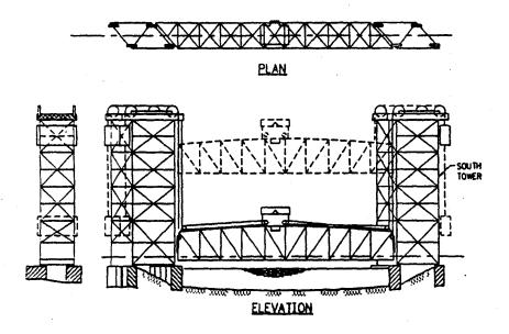
Figure 20-14 Vertical Lift Span with Power and Drive System on Lift Span; Due to Skew of Channel, Double Trunnions are Used To Place Counterweight on Back Towers
