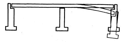
Figure 12-3 Differential Settlement Between Different Substructure Units
