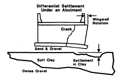
Figure 12-4 Differential Settlement Under an Abutment
