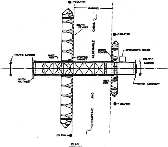
Figure 20-3 Swing Span with Unequal Span Lengths
