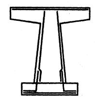
Figure 12-10 Primary Reinforcing Steel in Hammerhead Pier
