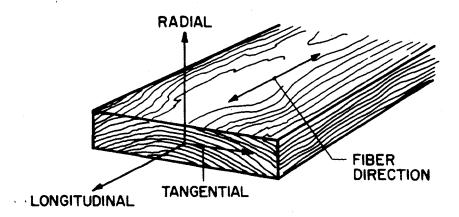
Figure 4-3 Three Principal Axes of Wood
