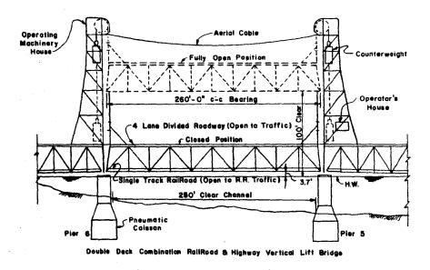
Figure 20-17 Outline of Double Deck Vertical Lift Bridge in Closed Position (Solid Lines) and Fully Open Position (Dotted Lines)
