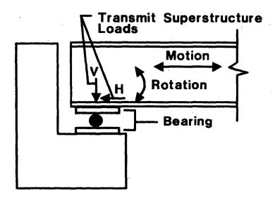
Figure 11-1 Functions of a Bearing
