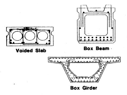
Figure 6-13 Prestressed Concrete Shapes
