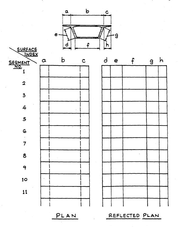
Figure 21-19 Form for Recording Cracks and Spalls in a Box Girder
