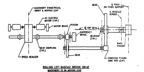
Figure 20-7 Rolling Lift Bridge Machinery (for One Quadrant) is Located on the Moving Leaf, which Rotates the Centerline Rack Pinion (Center of Roll) as it Rolls Open
