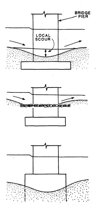
Figure 13-6 Local Scour and Local Scour Reduction at Bridge Piers
