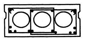
Figure 9-24 Prestressed Slab Beam Bridge Reinforcement
