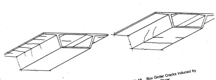
Box Girder Cracks Induced by Flexure (Negative Moment) Figure 21-11
