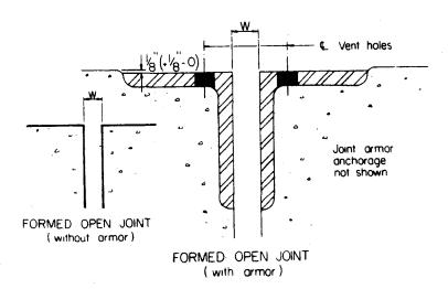
Figure 7-7 Formed Joint
