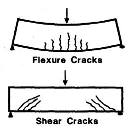
Figure 4-15 Structural Cracks
