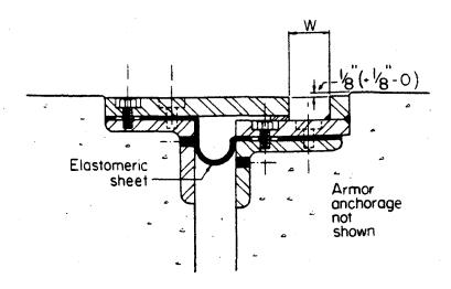
Figure 7-10 Sliding Plate Joint
