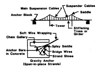
Figure 21-2 Special Elements of a Suspension Bridge
