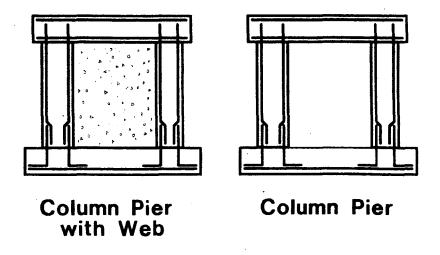
Figure 12-9 Primary Reinforcing Steel in Column Pier With Web and in Column Pier
