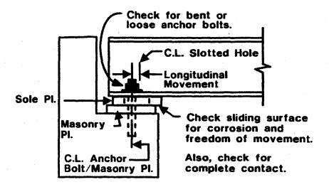
Figure 11-14 Sliding Plate Bearing Inspection Checklist Items
