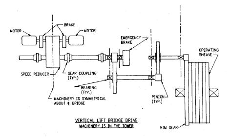
Figure 20-15 Vertical Lift Bridge Machinery is Located on the Towers, and the Rim Gears (and Operating Sheaves) are Rotated to Raise and Lower the Bridge
