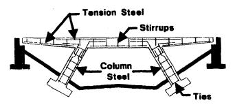
Figure 9-21 Reinforcement in Rigid Frames
