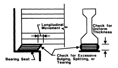
Figure 11-17 Elastomeric Bearing Inspection Checklist Items
