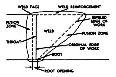
Figure 18-3 Groove Weld Nomenclature
