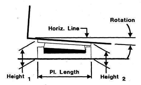
Figure 11-16 Angle of Rotation for Pot Bearing
