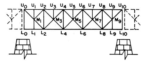
Figure 5-4 Sample Truss Numbering Scheme
