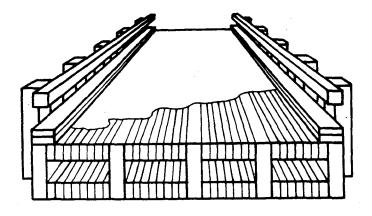
Figure 8-12 Stressed Box Beam Bridge (Source: Barry Dickson, West Virginia University)
