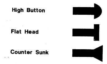
Figure 6-24 Types of Rivet Heads
