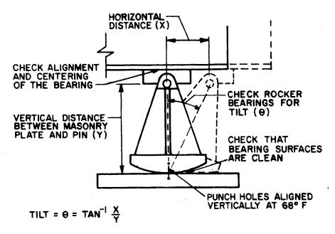
Figure 11-15 Rocker Bearing Inspection Checklist Items
