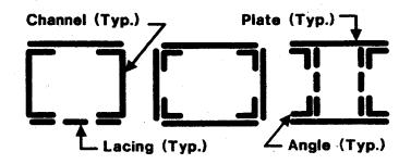
Figure 6-18 Riveted Box Shapes
