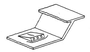
Figure 21-17 Box Girder Cracks Induced by Concentrated Loads
