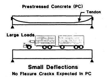
Figure 4-12 Prestressed Concrete
