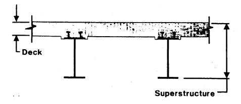
Figure 3-17 Composite Bridge with Concrete Deck on Steel Beams
