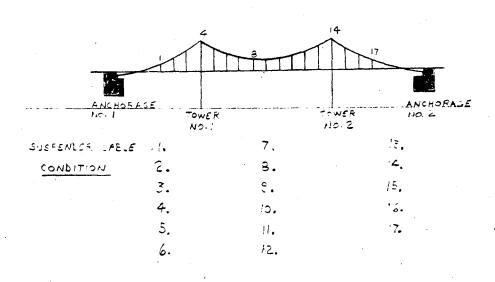
Figure 21-3 Form for Recording Defects in the Cable System of a Suspension Bridge
