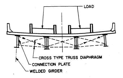
Figure 4-26 Out-of-Plane Distortion
