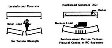
Figure 4-10 Reinforced Concrete
