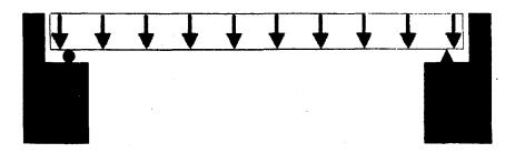
Figure 3-1 Dead Load on a Bridge
