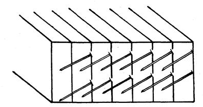
Figure 7-3 Section of a Nailed Laminated Deck
