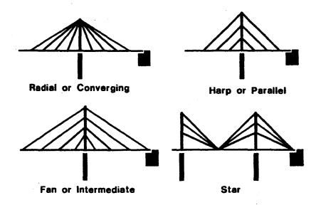
Figure 21-5 Longitudinal Cable Arrangements
