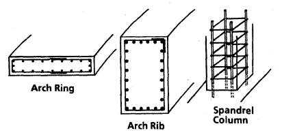
Figure 9-14 Open Spandrel Arch Reinforcement
