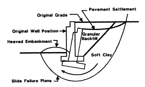
Figure 12-5 Lateral Movement of an Abutment Due to Slope Failure
