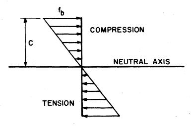
Figure 3-10 Bending Stresses
