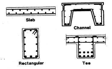
Figure 6-12 Reinforced Concrete Shapes
