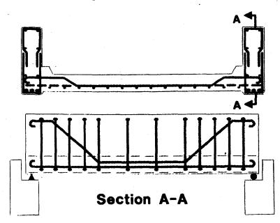
Figure 9-9 Steel Reinforcement in a Concrete Through Girder
