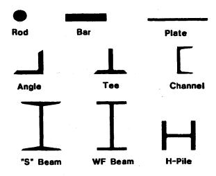
Figure 6-15 Common Rolled Steel Shapes
