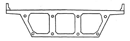
Figure 9-40 Multi-Cell Box Girder
