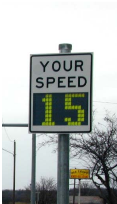
Figure 2. Example of a Permanently Installed Self-Contained DSDS Unit.
