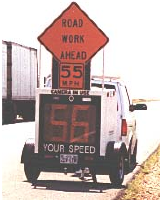
Figure 1. Example of a Portable Dynamic Speed Display System for Work Zones.
