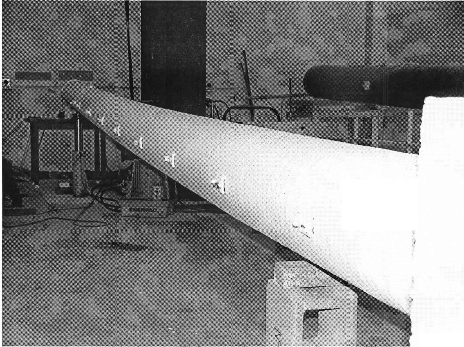
Figure 2.11 FRP pole deformed at 1 kips (4450 N)
