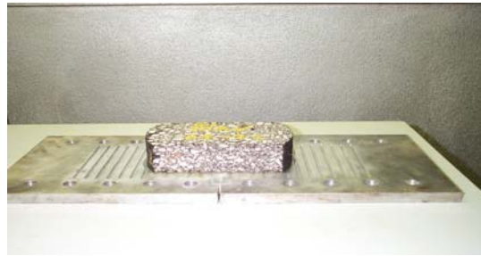
Figure 15. Test Specimen Glued to Plates.
