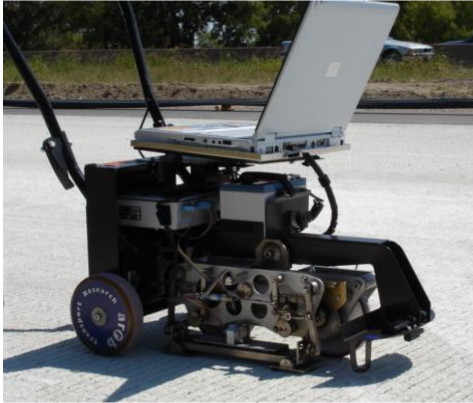
Figure 2-6. Walking Profiler Used to Establish Reference Profiles.
