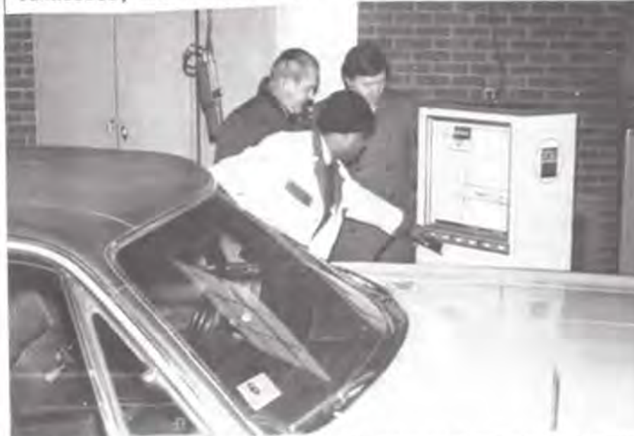
Curtis Bullock, D.C. Vehicle Inspection Technician, points to the reading on the dynamic front wheel analyzer, which gives an electronic readout of caster, camber and toe-in. With Inspector Bullock are Eldon Rucker, Acting Chief of the D.C. Office of Vehicle Safety Research, and Joseph Innes, TSP (right).
