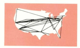
Electronic computers have been installed in the busier Air Route Traffic Control Centers in the Eastern States and comprise the world's only computer-to-computer air traffic control network. The essential facts of a pilot's flight plan are fed into these machines which automatically calculate his estimated time of arrival over designated check points within the Center's area of responsibility. The machines also print this information
