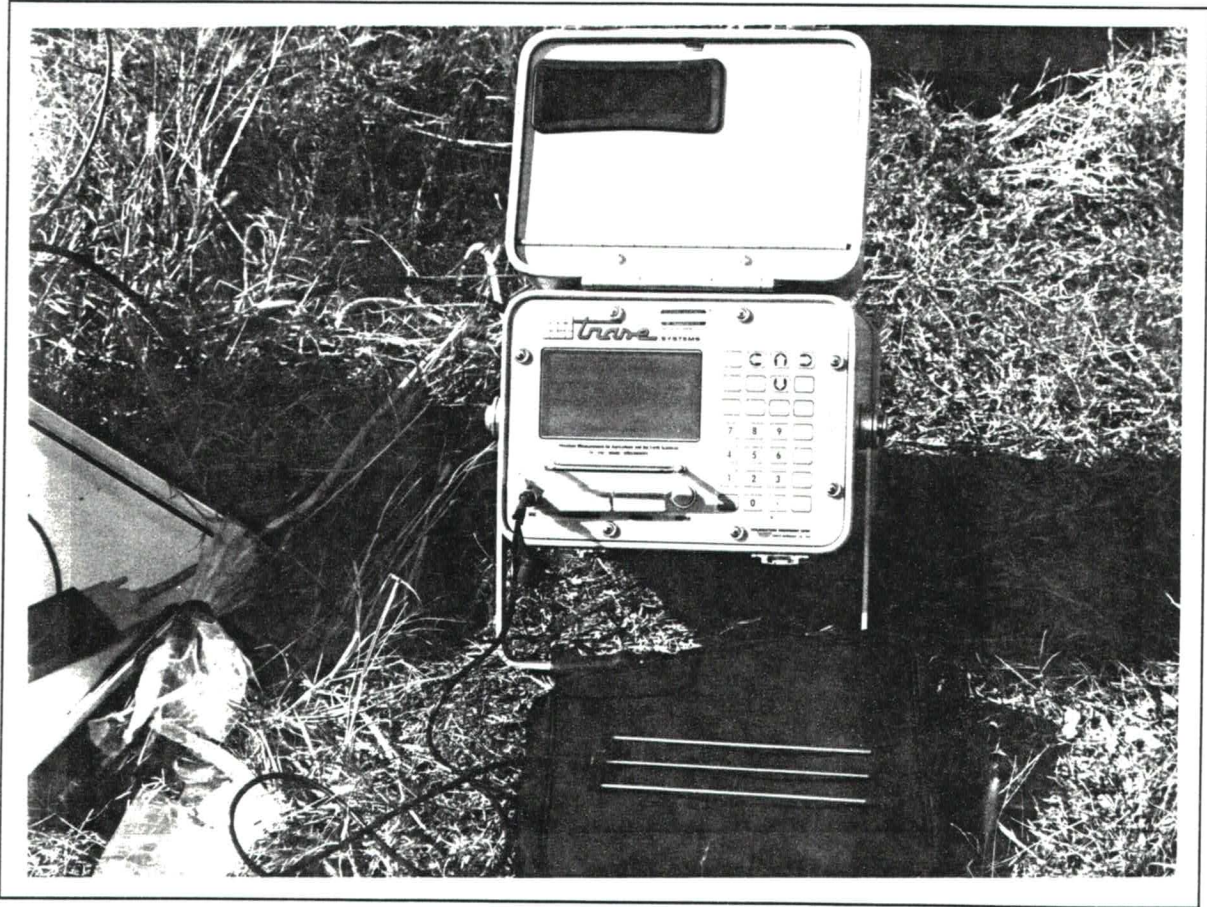
Fig. B-5 TDR moisture device and wave guide
