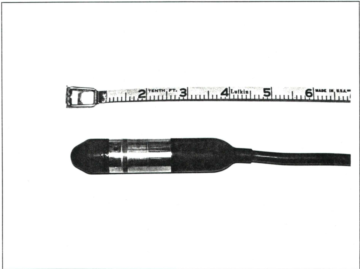
Fig. B-4 Pressure transducers
