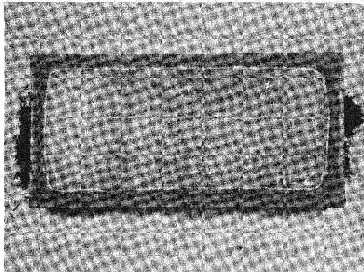
Figure 4.12 Surface abrasion effects due to the concrete bearing surface. The white line denotes the inner edge of the most severe abrasion.
