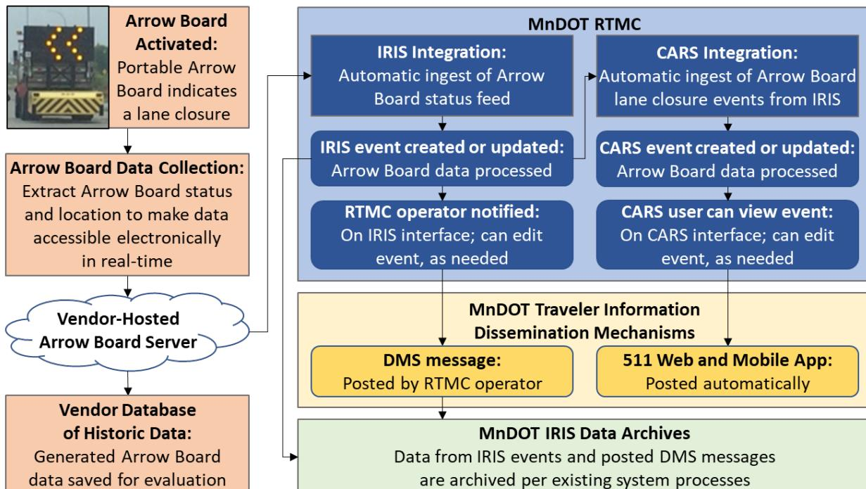
**Figure 2.7: Minnesota SAB project system data transmission pipeline**
