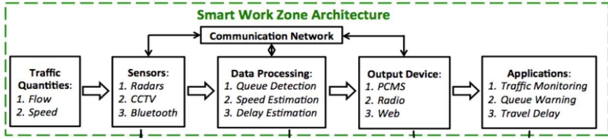
**Figure 2.1: Smart Work Zone Overview (Li et al., 2016)**
