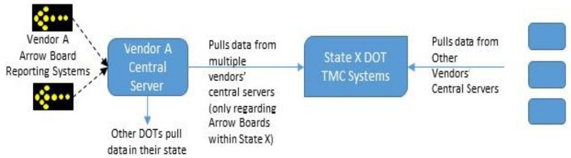
Another option is that DOTs would operate a proxy server to enable Arrow Boards to report directly to the proxy server, or to communicate via Vendor operated central servers. This would allow the TMC Systems to pull data from their own Proxy Server.
