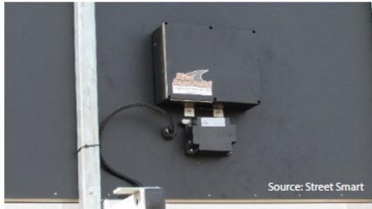
**Figure 2.8: MnDOT arrow board retrofit kit (FHWA, 2020a)**
