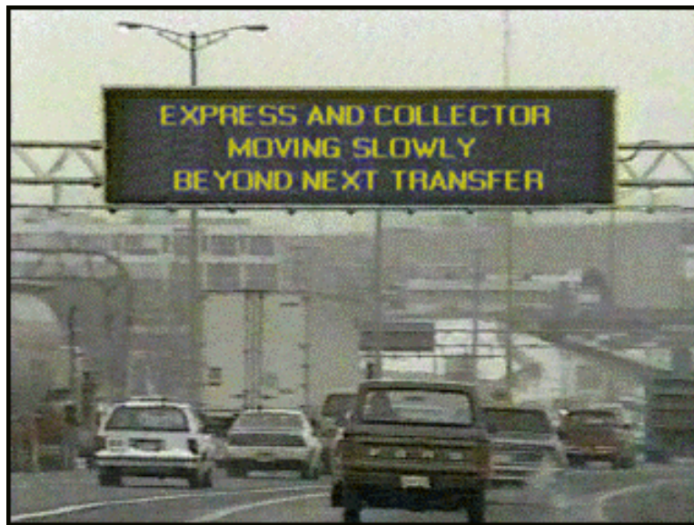
Figure 2-9. Large VMS Display in the Toronto Area. 28
