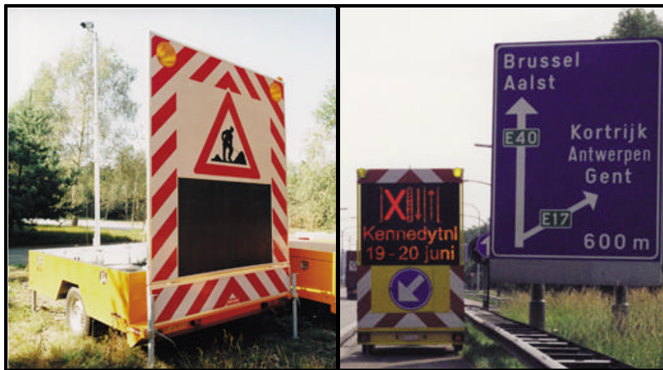
Figure 2-8. Trailer-Mounted VMS for Queue Detection and Warning. 27
