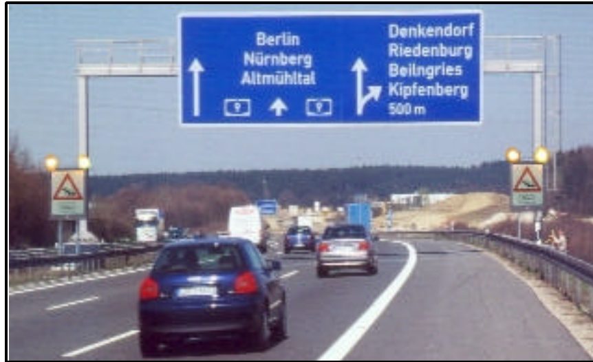
Figure 2-16. Mobile Traffic Jam Warning System on Autobahn 9. 38
