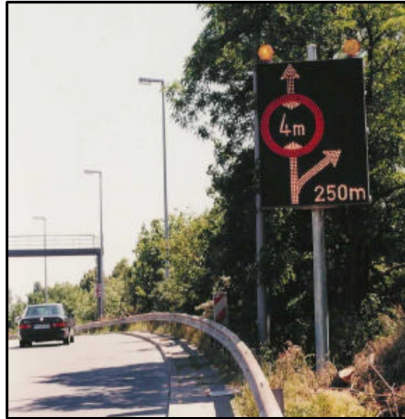
Figure 2-18. Small Roadside VMS on Autobahn 100 in Germany. 39
