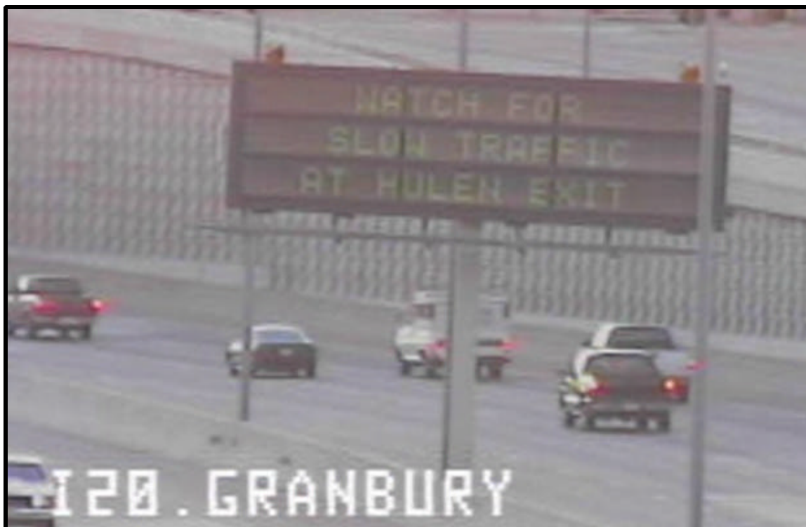
Figure 2-49. Warning Message on VMS About Potential Queue Spillback at the Hulen Exit Ramp. 94
