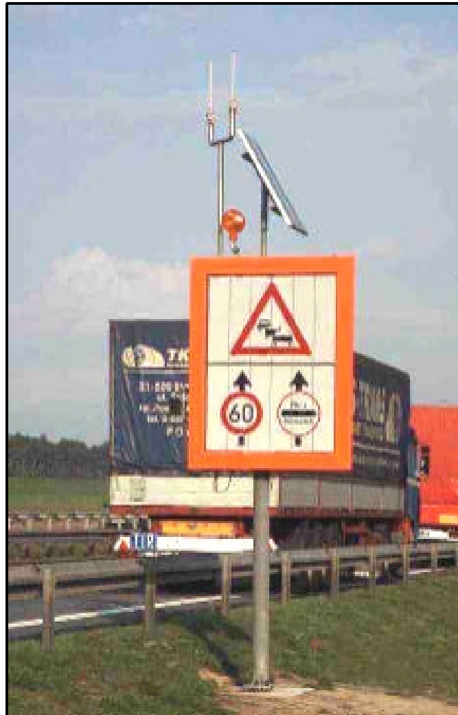
Figure 2-17. Mobile Traffic Jam Warning Sign near the Germany/Poland Border. 38
