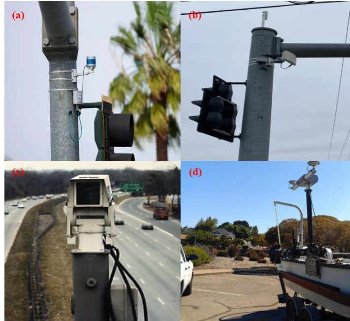
Figure 2. Examples of perception sensors used in transportation: (a) automotive LiDAR unit [10], (b) automotive radar sensor [11], (c) automotive camera module [12], and (d) sonar sensor [13].
