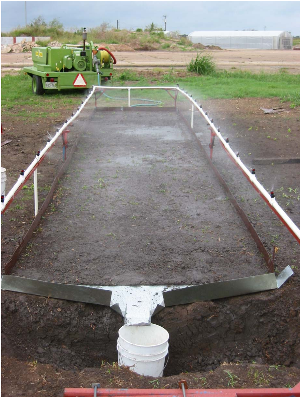
Figure 8. Artificial Rainfall Simulator.
