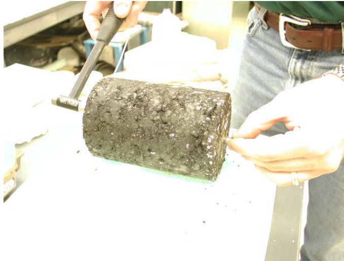
Figure 31. Black Base Specimen Tested for Seismic Modulus.
