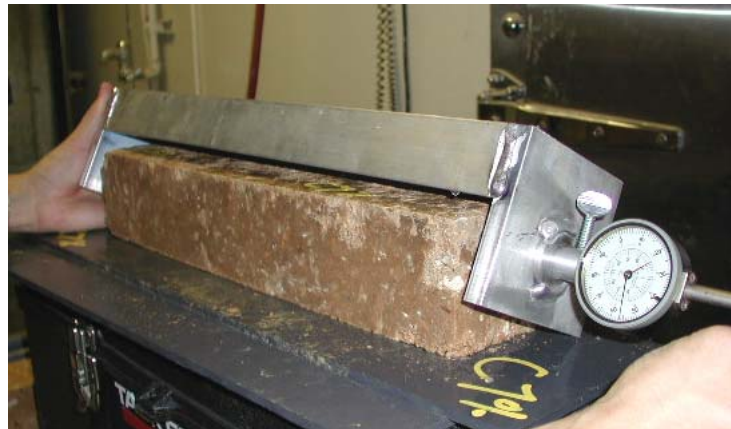
Figure 28. Shrinkage Measurement in Progress.
