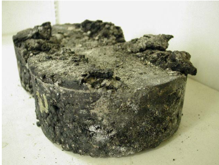
Figure 39. Black Base after Hamburg Test.
