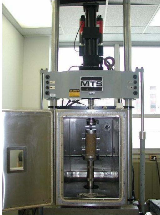
Figure 26. Resilient Modulus Test Setup.
