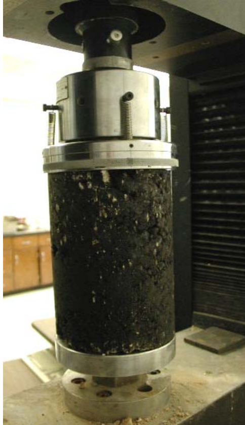
Figure 30. Black Base Specimen in Compression Test.
