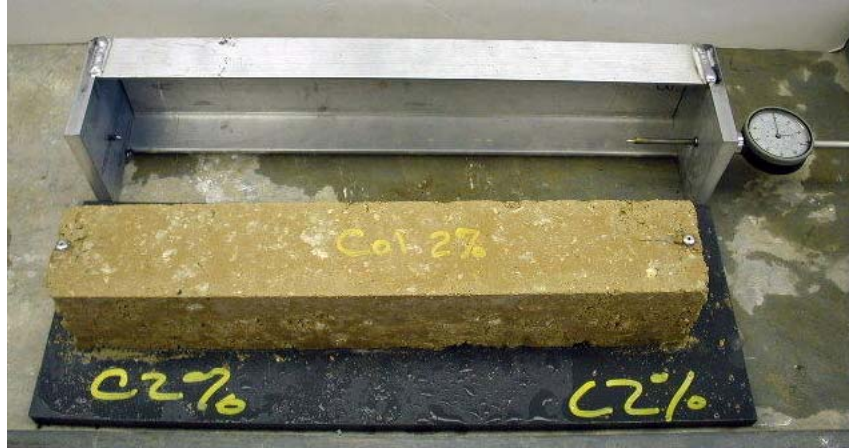
Figure 27. Beam and Measurement Device for Shrinkage Measurements.
