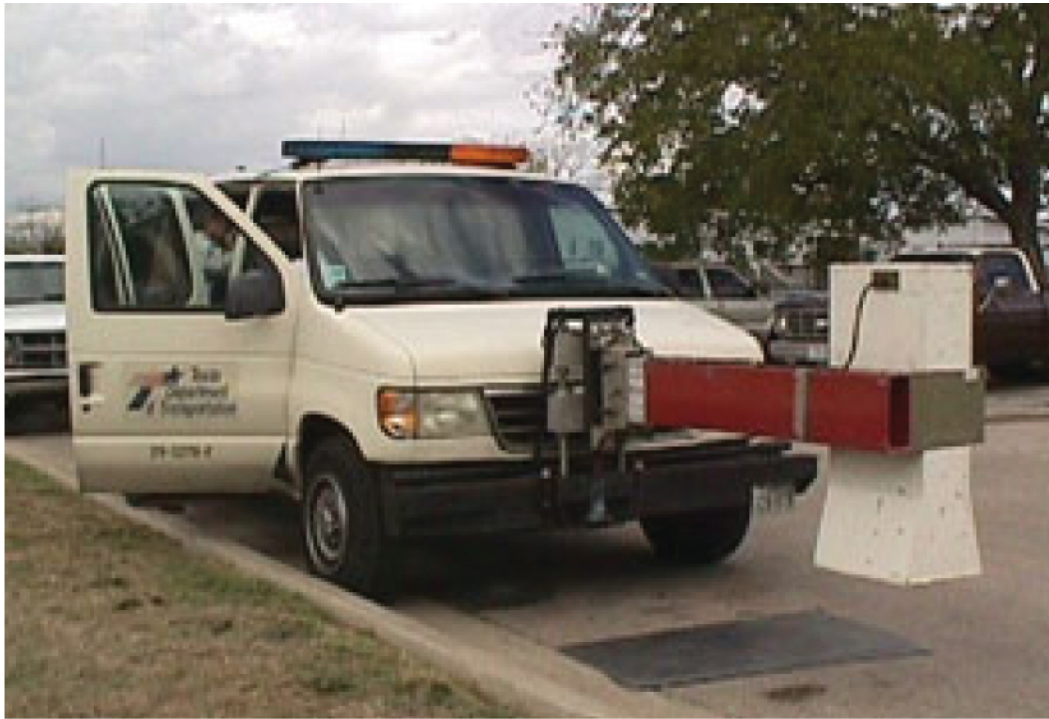
Figure 2.4 Ground Penetrating Radar Equipment Mounted on a Vehicle
