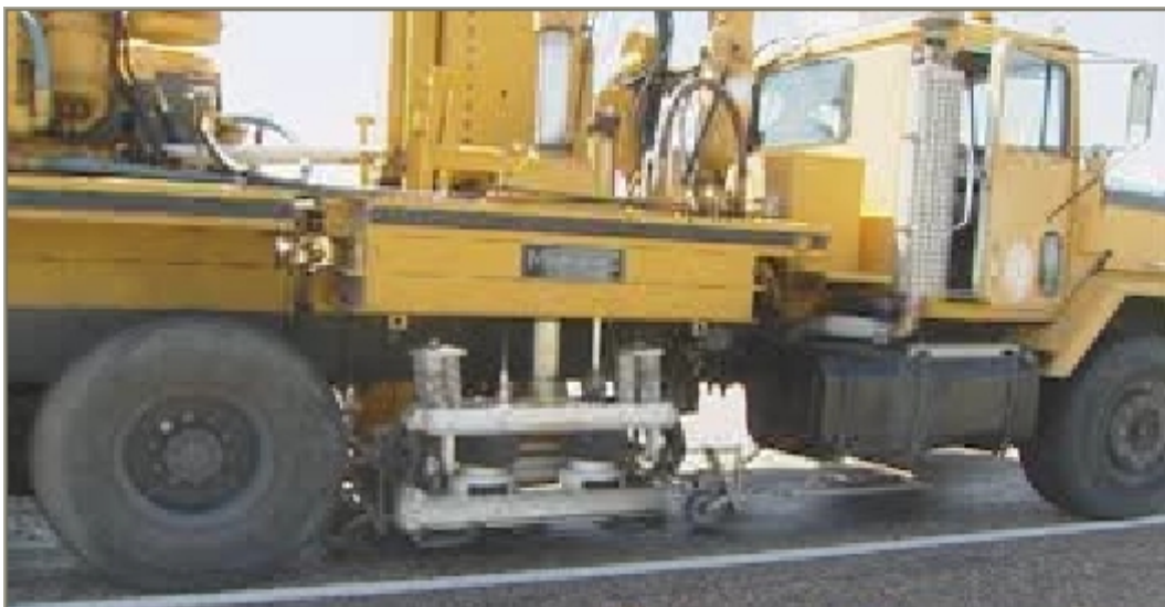
FIGURE 3 Rolling Dynamic Deflectometer
