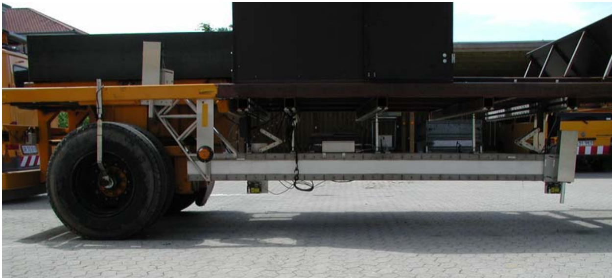
FIGURE D. 1 Danish HSD Trailer Showing Beam and Sensor Arrangement (Hildebrand, et. al. 2002)
