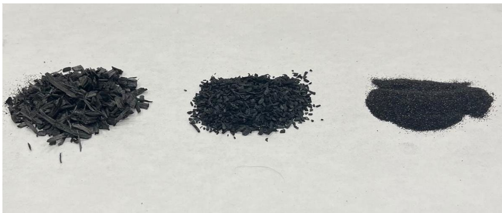
Figure 2.4 Images of a representative black ash biochar (525 °C HTT) product in three different sizings. As-produced (left). -10/+20 mesh (center). -60/+270 mesh (right).
