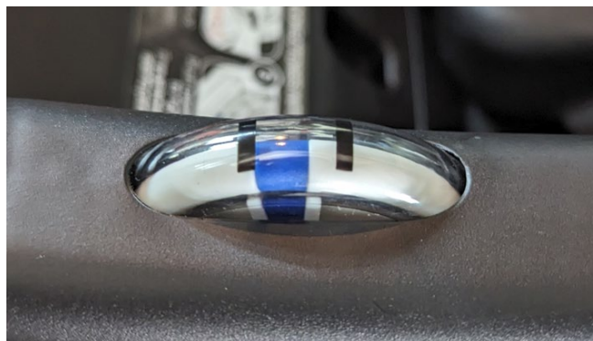
Figure 4: Bubble level indicator on a CRS. The manufacturers' instructions indicate that the CRS should be positioned such that the blue indicator is between the two black lines.
